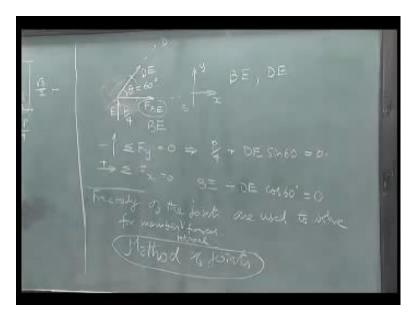
We have a cut here, this is E, we have B over here, we have D over here that these two members have been cut, there is an external force acting on it equal to P by 4. Since, we have cut here, we will be exposing an internal force in each of these members, that act along the axis of these members. I tell you in a moment as to what direction force I have to insert over here, for now I will just put the internal forces to be like this.
