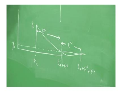
In the last part, namely a both impulses with which we will continue in the next class. We will just introduce the subject and carry forward in the next class. And what is the impulse, when we talked of over pressures, what we are basically considering is, we are having a blast wave, which is created. And the effect of blast wave is to create something like a pressure, which crushes.
