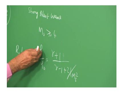
And we were able to determine, what did we determine, we said as R S by R 0 increases. We have P S minus P 0 divided by P 0, which keeps following down, which rapidly changes. Well, we did this for a strong blast or a strong blast wave, what do we mean by a strong blast wave. In the field, near to this, that means in the region very near to the source. Wherein, the much number of the shock wave, which is from is quiet large, may be typically greater than around 4.
