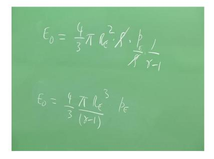
And therefore, if I write the value of the energy, which gets release, let us put that down. We get therefore, e not is equal to 4 upon 3 into pi into R E cube into grow into P by row into 1 over gamma minus 1, rather row. And row get cancel and this is the pressure of the explosion. Let me call it as P E to distinguish from the ambient pressure P naught. And therefore, I get the value of E 0 is equal to 4 upon 3 into pi R E cube into P divide by gamma minus 1.
