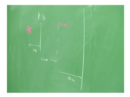
In other words, we are talking of a situation, wherein, some energy is released over here. All of sudden instantaneously, the energy releases is 70 Mega Joules, the ambient pressure at which this energy release is 0.095 megapascal. You know, 0.095 is very near to 0.1 megapascal and this might be at a slightly increase attitude. And now, I am interested in finding out, what is the magnitude of the over pressure, may be, I deposit this energy at a distance.
