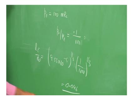
In the limit, now I tell myself, in the limit, were P is very large number. Maybe, the explosive is such that, I have intense pressure, pressure tends to infinity, when P E tends to infinity. Well, the value of R E by R 0 is that; that means, R E by R 0. When, I have a high pressure explosion tends to 0. Well, I am getting the point explosion like, what we are been considering, we do not even need to consider the effect of R E wave, when the pressure is very high.
