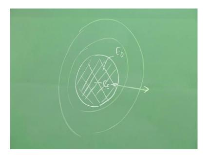
In the finite volume, if an energy is released, what is the effect on the value of the over pressure. And for that, we tried to again tell ourselves, well simplify the problem. We tell ourselves; well I am interested in say, a spherical volume as sphere. Let us say, that radius of the fear is R E. And the energy is gets liberated in this particular volume. This is where, now I say the energy is getting liberated.
