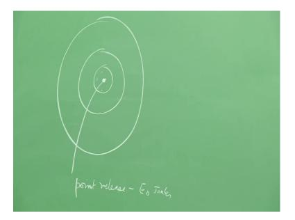
All what I tell now is, well I have been able to get this figure, which I say is for an explosion and what did we consider. We considered, when some energy is release that a point, let us say or energy is release, we told ourselves well as spherical wave propagate and spherical blast wave propagates out. We did not really consider the dimensions of this particular point, at which the energy is gets liberated.
