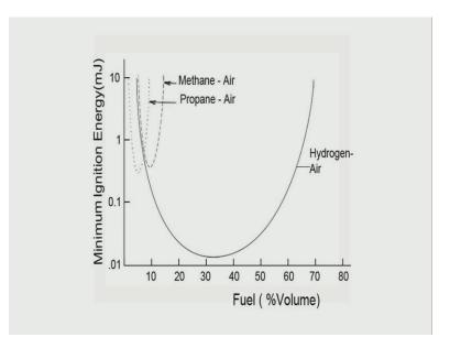
Therefore, we go for the we say that these are the minimum ignition energy as a per percentage of volume of fuel divided by the volume of mixer. We find well Propane air has a very narrow range and the upper range was 9.5 and the lower range was around 2.2 well the stoichiometric around 4. And when we talk of Methane well; my Methane has a lower value of the has a yes higher value of the percentage fuel in the volume of the mixture.
