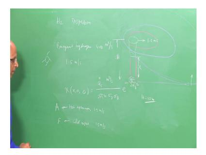
Such as, hydrogen gas and its dispersion well the type of equations what we use the way we do the problems remains the same. Therefore, let us consider the specific example of point Hydrogen being released accidently at the rate of 400 meter cube per second from a stack. You know may be there is a plant which is generating, may be by there is some excess Hydrogen, may be some it is getting released at this particular rate at some instance of time.
