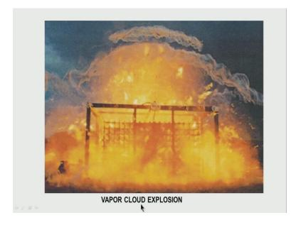
Well, this is what really happens? what happens is a vapor gets generated, the vapor burns or rather you gave hot vapor which rapidly burns forms a blast wave, and this is what happens in these oil tanker explosions, namely a vapor cloud gets generated.
