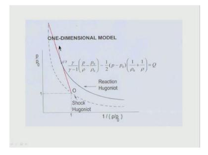
We are saying in the 1 dimensional model, we had the reaction Hugoniot over here. We had the initial point over here. We drew the Raleigh line, this is the upper point at which it was tangential, we called it as C J point, over here we said well this is the steady state velocity of a detonation.
