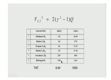
I show in this particular slide we use this expression V C J square is equal to 2 gamma square minus 1 into the heat release and whether we use it or do iteratively, we do iteratively we get for different gaseous mixtures stoichiometric mixtures for which the initial condition is 1 atmosphere and initial temperature is 298 kelvin.
