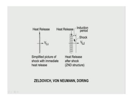
And once we are able to translate it into the structure of a detonation, we find well I have a shock here, I have a induction period over here in which may be there is not much heat released at all. But it is at a high temperature and followed by a zone of reactions in the, in the picture what I had when I talk in terms of a Chapman Jouguet detonation, I just presumed that the heat is getting released. I never looked at this mechanism of an induction tank heat being released a little later.
