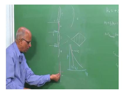
It is not a single shock wave we have something like an incident shock, we have a mark shock, we have an incident shock, we have a mark shock and we also have transverse waves which move behind it. We have these transverse waves moving here and these things the triple point where in you have the transverse waves and the shocks combining these are known as the triple point.
