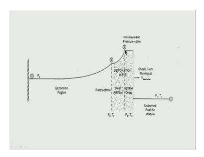
If I try to look it in a slightly different format well I have the initial temperature here, a shock moves. I have a pressure which is formed here I have the pressure behind the shock we said is higher than the detonation pressure which is coming over here. And the gases further expand over here.
