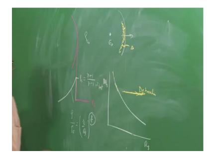
You had a shock front over here. We said well, at the front what happens you have the initial density is row 0 in the unburned medium over here. You have the density increased to row s, and the value of row s was gamma plus 1 divided by gamma minus 1 for a string shock, for a weaker shock well, I have to over M s square over here.
