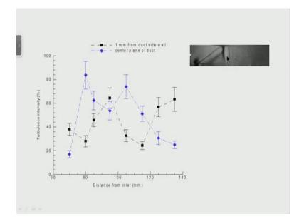
And these things what they do is, they create high intensity turbulence, know because you have flow directions being changing, you have slip streams over here, you have very high intensity turbulence over here. And this high intensity turbulence and also the length scale of turbulence also increases behind the leap shock wave, which is in the unburned gases.
