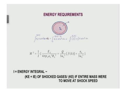
And therefore, now we can write the expressions down. We found, yes we wrote an expression for chemical energy release, when all the chemical energy is released. But now we find well, there must be a distance that means, shock is over here it takes a definite time for chemical reactions to occur.
