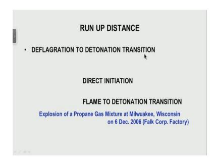
And to just sum up well, the run up distance is for deflagration to detonation transition. It is different from direct initiation wherein, the energy source from directly at detonation. The initiation source forms the flame, which later transits to a detonation.
