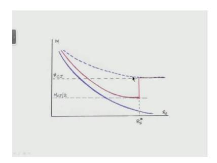
Well, I have mark number versus the distance, if the energy release is low well, I by the time a core of chemical reactions is formed, the shock wave has decayed to low velocities and it really cannot form a detonation. If the energy release is large E 0, we find this that, this is the direction of energy release, if the energy release is large well, I am able to form a detonation.
