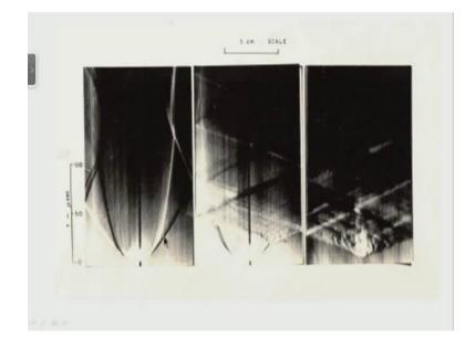
I can also show it in a sheet picture wherein, maybe when you have the shock, that is the blast wave is over here, it travels forward. You have the chemical reaction zone which are over here, chemical reaction zone over here, blast wave over here. You know that too keep on increasing distance and therefore, the energy is insufficient to form a detonation kernel of some minimum size.
