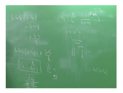
Being this the value of S u is we said is equal to 0.5 into u h so much we are talking of in metres per second. Therefore, the thickness of the flame is so much metre. Well, the unit is all right and therefore, we say the thickness of the flame is typically around 10 to the power of minus 4 metres or which is around 0.1 metres.
