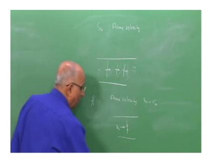
You will find people talk in terms of flame velocity, is flame velocity same as the combustion front, which moves or we say the value of the value of S u, which we said is the velocity with which the unburned gases are moving towards. The front is it same as the flame velocity. Let us go back and look at a particular experiment.
