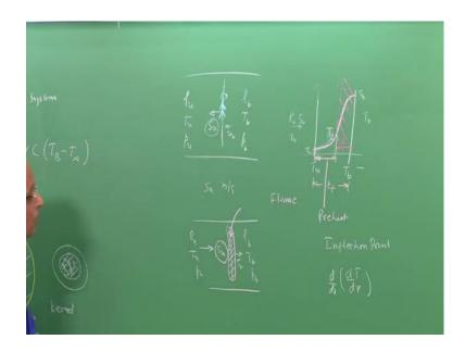
Let us say, I have a zone of combustion. For I also say, I have a pipe or a some particular medium in which, well, I have the unburned gases unburned gases are at density rho, which is unburned. Well, they are at a temperature T u, which is a unburned gas mixture, and we can also say, well the pressure of the unburned gases is p u into this unburned gas mixture. Like I have the unburned gases here, unburned gases here into which a combustion wave propagates or the zone of reaction propagates.
