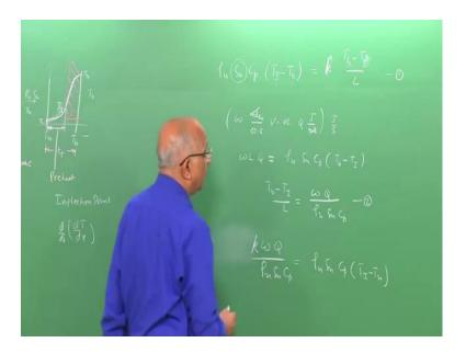
Therefore I say, well the mass which is entering is rho u into S u into 1 that is the, that is the mass flux into 1, which is the mass, which is entering. Let us for the present assume it is at constant pressure C p; we will rectify this assumption a little later. Therefore, this is the thermal mass over here, and what happens in this zone.
