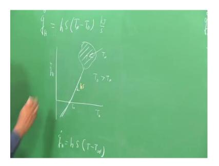
We tell that the heat transfer, and let us put the same thing the rate of heat transfe we say q dot H is equal to, it is depends on the temperature difference. We have T ambient minus T naught, and what drives it is the heat transfer coefficient into surface area? We say so much kilo joules per second is the heat transfer over here.
