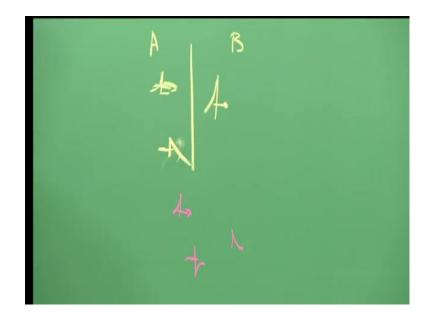
Therefore, we tell ourselves well based on this expressions I also tell myself that when the impedance of two media A and B are such that when a greater than b, I have a compression reflected as a compression back over here. Something which gets transmitted is even of greater value greater pressure which gets transmitted over here. The movement when I talk of the impedance of medium a being less than or impedance of lets us say medium of the second medium B being very much less than this.
