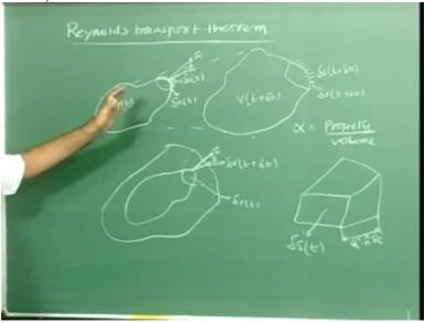
Where you are completely working with the arbitrary shape control volume, which is not fixed to any coordinate system, okay and this is a very interesting approach. So here what we do is we consider a control mass essentially a system that means, we are considering fixed packet of fluid with a given mass and tracking it with respect to time. So if you assume that there is a
