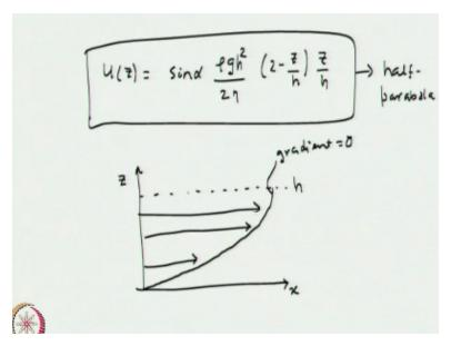
So, this is z this is x along the flow direction in the inclined plane and this is perpendicular to the inclined plane. And let us say we are talking about this as the film height okay this is the film height. So, the velocity is going to look like this like a half parabola and right at the surface it is going to be okay here the gradient is going to vanish the gradient=0 and this is the general velocity how it is going to vary along h.
