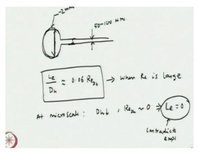
Which is typically in a rounded shape and then the flow gets into the microchannel and these are typically of the order of you know a few millimeter and these are of the order of the say 50 to 100 microns right. So, the height here in this plenum and here in the channel area they are the same but if you look at the other direction this is large as compared to here. So, in this direction in the horizontal plane the flow is uniform.
