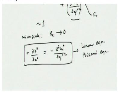
So, micro-scale the Reynolds number would turn to 0 okay. So, we will have an equation so the entire left hand side will drop off. So, what we would have here is you know –delta p star /delta x
