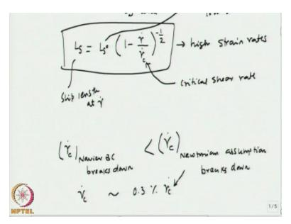
Ls can be written as Ls0\*1- this is the strain rate gamma or gamma. Critical \*-1/2 ok so this is how the slip in the is going to vary at high strain rates. Okay when this is going to happen when the shear rate or the strain rate is higher than the gamma critical okay. So, this is the critical shear rate this is this is going to be this is going to be the slip length at certain gamma certain strain rate and this is the slip length at low shear rates which is constant okay.
