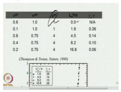
If you look at this table here this term is representing the ratio between the inter atomic distance to intermolecular distance when this ratio is 1 the slip length is 0 okay and when this ratio is becoming 4 the slip length could be as high as 16.8 times than the intermolecular distance in the fluid. Okay so that is what we learn from this molecular dynamics simulation data now we know that the slip length is not a function of the shear rate or the strain rate.
