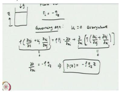
So, the first example we will take is the hydro static pressure this will find for a fluid in mechanical equilibrium. So, this is the simplest case possible where we will try to derive ore we can find out the hydrostatic pressure for a static liquid in a container okay from Navier Stokes equation here the fluid is stationery so the velocity will be 0 and the only terms that will exist is the pressure term and the body force term okay.
