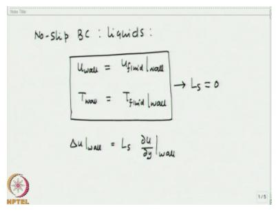
So, no slip boundary condition or liquid you can write that u at the wall will be=u fluid at the wall. So, velocity of the wall is velocity of the fluid at the wall. Similarly, T wall is temperature of the fluid at the wall. So, this is the no slip boundary condition for liquids so what does it mean it means that our slip length in this case is 0 right we can generalize we can write delta u at the wall is Ls\*delta u/delta y at the wall.
