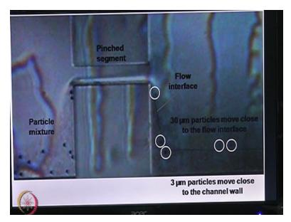
We are also doing experiments the particle setting this is a mechanism called pinch flow fractionation where we use a pinch segment to pinch a particulated sample with pure fluid and based on the principle that particles tend to move along the stream line passing through the center of mask the bigger particles will be closer to the center line. And the smaller particles will move close to the wall. And that is how we will be able to sort particles using pinch flow fractionation.
