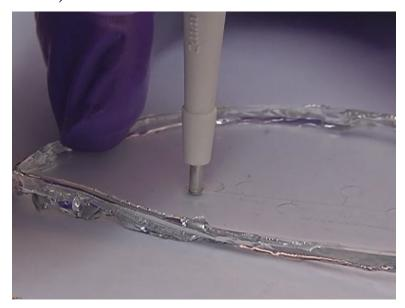
Okay so the projection that was on the master has been formed by the channel on the PDMS. We are going to bond with the glass to seal the channels and you know to enable interconnection between the external fluid supply typically syringe pump and the channels in the microfluidic chip. We are punching the interconnection holes you can see the punch which we are putting it through the PDMS layer to create the interconnection.
