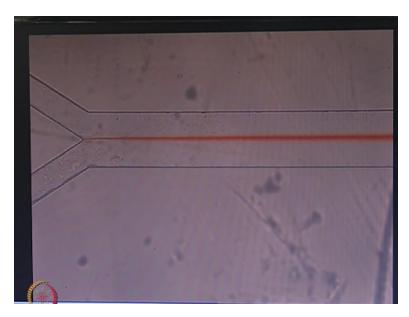
So this was the video that the experiment that we have running where 2 fluids being mixed 2 colorless fluids are being mixed and as they come in contact with each other a diffusion zone is developed and as you can see the width of the diffusion zone increases along the flow direction okay.
