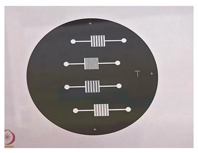
As I was telling you the first you know study the device structure that we want to fabricate and then we come up with the mask layout and we get the mask printed that you can see here okay and this mask is used to follow the photolithography process to make a master which you will be using to make the PDMS based microfluidic device.
