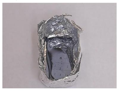
So, we have prepared and aluminum boat and inside that you can see the master and now we are going to pour the PDMS onto this master. So, the thickness of the chip would depend on the quantity of the PDMS that we pour on the master you can see some bubbles getting trapped during the pouring process which is be removed during the baking that you do in a vacuum oven.
