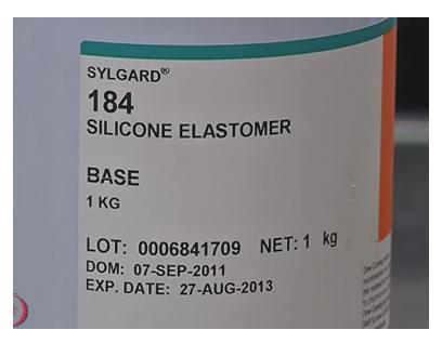
So, this is the you know we have using the silicon master to make PDMS microfluidic device so to make PDMS microfluidic device there are 2 components 1 is the base which is the silicone elastomer which you see it here.
