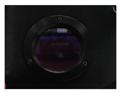
So were going to treat the PDMS and the glass slide surface with the oxygen plasma for about a minute and you can see the oxygen plasma the correlation is light blue color that you see okay.So, once the treatment is over we take out of the plasma chamber and bond them okay after the glass and PDMS are treated.
