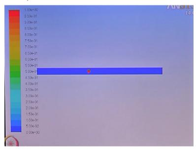
So, this is a simulation of the motion of a droplet in a microchannel that we are trying to do here and were trying to predict the additional pressure drop that we encounter in the presence of a droplet as compared to in a case where we do not have droplet present in a channel okay.
