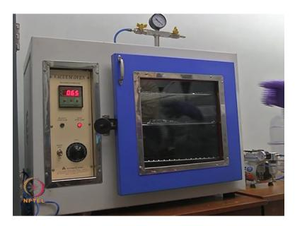
Okay so after pouring the PDMS onto the silicon master to remove the air bubbles and to cure the PDMS we are putting whole setup into the vacuum oven. So, the temperature is 65 degrees C which is used for the curing of the PDMS. So, once the PDMS is cured for a duration of 3 hours at 65 degree C we take out from the oven.
