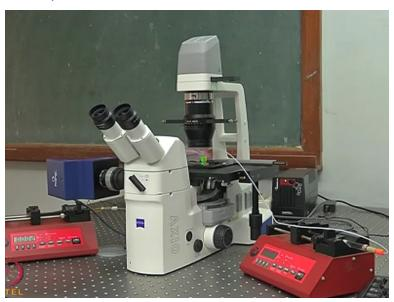
So here you can see you are doing an experiment on mixing mixing 2 fluids in a micro channels as you can see we have 2 syringe pumps driving 2 different fluids equal flow rates and so the 2 fluids still mix going to be a diffusion zone which is going to be developed.
