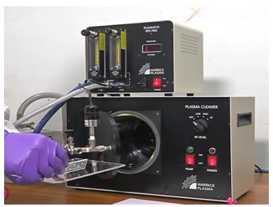
We take it out of the chamber and put the PDMS is on the surface facing down on the glass slide.
