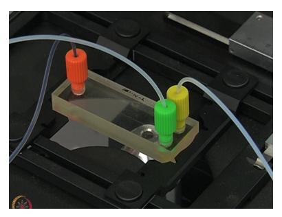
So, here is the microchip that way of using for the experiment and you can see there are 2 inlets and 1 outlet and the inlet fluidic connection is by quarter 28 unit thread and we have these fluidic threads also connected to the capillaries and which are threaded on to the fluidic hole or the connection.
