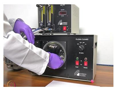
So, were going to bond the glass slide with the PDMS, so they have put in a quad surface and put inside the plasma cleaner.
