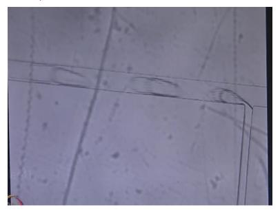
This is an experiment generation of micro droplets in micro channels as you can see the continuous phases trying to shear the discreet face where discreet droplets being formed in micro channels.
