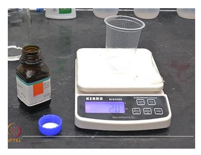
We are mixing it with 2 grams of the curing agent, so we have the base and the curing agent 10:1 ratio.
