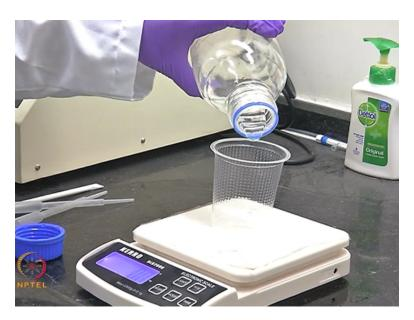
So, we poured this is the basis which we discuss and we use 10 parts of the base and mix it with 1 part of the curing agent. So, this is 10 part of the base that we just poured on to the glass we can use a plastic disposable plastic glass.
