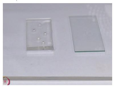
Okay so after punching the holes we are going to bond the chip with a glass slide you can see that after punching the holes the PDMS has been trimmed off to the shape of the chip. And it is going to be bonded with the glass slide as you can see here and for that were going to treat both the surface of the PDMS and the glass using oxygen plasma.
