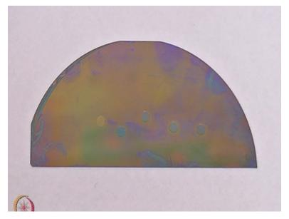
After we do the photolithography so this is the master that we have fabricated using the photolithography process so it is basically an estimate pattern and to the silicon wafer which is an issue is a negative photoresist. So it is patterned on to this silicon wafer using photolithography.
