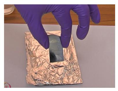
So, this is the master that we have so it is a part of the master cut out so many times we have many different chips on a single wafer. So, this is part of the way for it as one single chip and we are going to pour the PDMS mixture that we have prepared onto this master.
