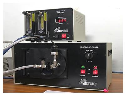
So ,after the pressure required pressure is reached plasma power is switched on and the setting is at the medium level with slight adjustment of entrance of the oxygen into the chamber we can create the plasma.
