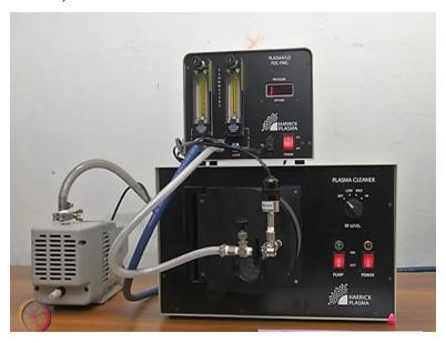
So, this is the plasma system that were using it has basically 3 different parts, this is the main component this is the plasma chamber inside which you will have electrodes and you know the top one that you see there is a pressure gauge it also has a flow meter. And on the left you would see a vacuum pump it is a special vacuum pump it should be noted that since were dealing with the oxygen plasma.
