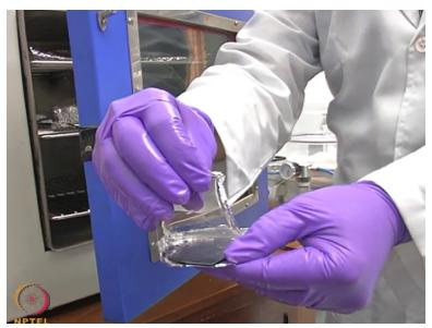
One such PDMS setup which has been cured for last 3 hours you can see it here that is solidified. Now we are going to peel the PDMS off from the silicon master. So. we can see that it has solidified and now were going to peel the PDMS from the silicon wafer peeling has to be done from 1 end and it has to be very gently pulled out. So you can see that the pattern that was on the master has been printed onto the PDMS.
