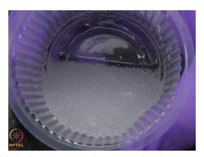
So, that is how it looks after the base and curing agent are mixed thoroughly there are only a lot of bubbles that you can see that trapped so it now we are going to do the degassing to remove these bubbles.
