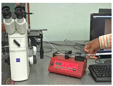
So this is the syringe pump the fluid into the microfluidic chip we have a glass tight syringe and this since pump is going to be driven by the stepper motor and so this fluid is going to be pushed and going to go to the chip using this capillary.
