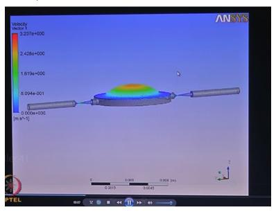
So, this is a pressure electric actuated valve less micro pump that we are trying to simulate as you can see there in the forward stroke as the membrane moves up the fluid comes into the chamber more as compared what it goes out. And in the reverse stroke when the membrane goes down more fluid goes towards the exit outwards toward the outlet as compared to what goes out through the inlet.
