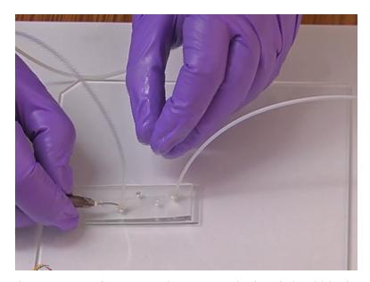
And we apply gentle pressure so it very gentle pressure the bond should be irreversible okay. So the PDMS is irreversible. Now the capillaries will be bonded to the chips on the punch whole areas and so the capillary is inserted into the holes and we glue it around. So, that is how the external fluid is going to be supplied to the chip.
