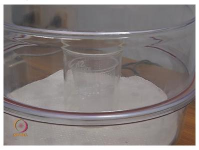
So, this is the vacuum desiccator which is connected to the vacuum pump and we are going to do that the degassing of the mixed base and the curing agent that we had seen earlier after all the bubbles are removed from the make sure this is how it is going to look like is a transparent solution with no bubbles present okay.
