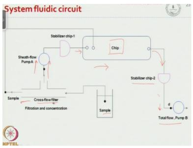
So this is the system fluidic we have sample coming in here, and it gets into a cross flow filter which basically filters the pure fluid which is used for focusing the sample. And here concentrated sample is coming in which is being focused by the pure fluid, so that all the detection is happening here, and then the particles exit okay. And this the fluidic transferred is controlled by the 2 different pumps.
