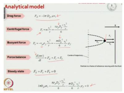
So before we designed the device you know the in analytical model was developed to look at the physics based on which this particular separation is achieved, so there are different forces that act on a particle that is going through the trajectory of the spiral path. One is the drag force which is given by the -3 pi\*the diameter of the particle mu\*vr, mu is the viscosity, and vr is the radial component of velocity.
