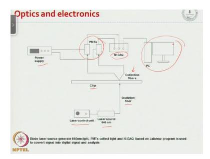
So this is the general arrangement of the experimental setup, we would have a chip, and we have already shown the fluidics circuit, here we show the optoelectronics, so here the laser control unit is arriving a laser source at 640 nanometer, this is the excitation fibre, and these 2 are the collection fibers we are collecting light and they are taking it to photomultiplier tube, which you know driven by this power supply.
