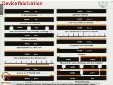
So after the simulation the device was fabricated, so it is fabricated based on a combination of you know photolithography and bonding. So it starts with a PMMA wafer, cleaning with oxygen plasma, and then the interconnectors where micro-milled using micro-milling, and then followed
