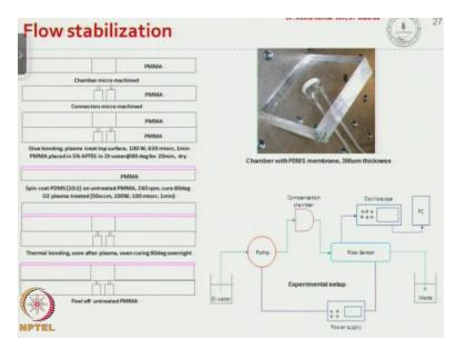
So this is the fabrication approach that has been used to fabricate this flow stabilizer chip.
