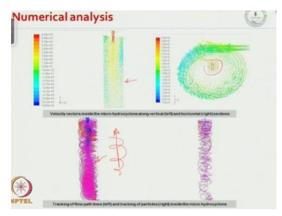
So here this shows the solution here this is the numerical simulation, here you can see that the particles have a tendency to go and follow the helical path, and it has the net downward velocity as you can see, and the liquids have a net upward velocity at the center. So this is confirmed by the tracking lines as you can see the particles are spiraling down as it goes okay, so it spirals down and the liquids are going up at the center.
