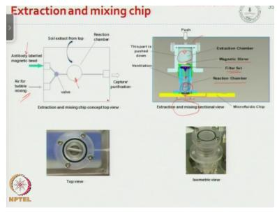
So this is the extraction chip, it has the plunger arrangement so you know here the top cover is taken out and the soil and buffer is introduced into the chamber here, and inside the chamber we have a magnetic stirrer which is driven by a motor underneath the chip, and this magnetic stirrer stirs the buffer and the soil solution. So after the soil buffer solution is mixed well then this plunger is pushed down, so here we have a filter set.
