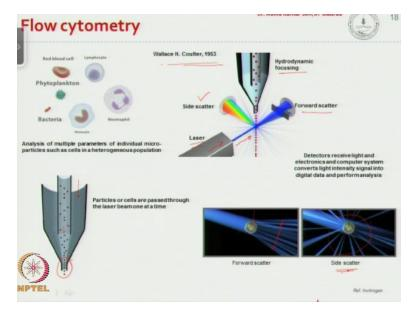
So this is the method of flow cytometry that is used for detection of microparticles, so different microparticles like blood cells, phytoplankton's, bacteria they can be all detected using micro flow cytometer. So this is the principle of the Coulter flow cytometer as you can see here, it basically has got 2 components, one is the fluidic component, the other one is the optoelectronics.
