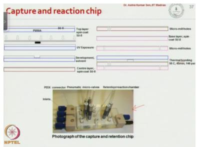
So this is the fabrication process how this capture reaction chip was fabricated, and it was fabricated based on a combination of photolithography and micro-milling followed by thermal bonding. So this is the chip that you can see here.
