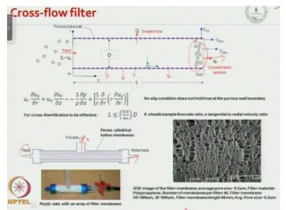
So here as we discussed there is a cross flow filter being used for filtration of the sample and the sheath fluids, and this cross flow filter basically uses a you know uses an array of hollow cylindrical porous membranes, where the particles can come in and the sheath fluid can exit around the perimeter, and the concentrated particle exit at the other end. So that is how we can bring in sample and concentrate the particle and simultaneously collect the pure fluid.
