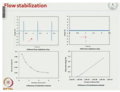
And here we show that by using the flow stabilizer chip that typically you know oscillating flow becomes steady with the time, which is essential for flow cytometer applications.
