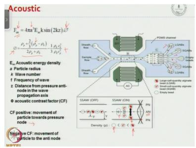
Here, we talk about acoustic based particle separation, the acoustic based particles separation this is the acoustophoretic force which is the function of size and it is also depends on the acoustic contrast factor phi, and phi is a function of the density of the particle and the density of the medium okay. Now the direction of the acoustophoretic force is dependent on the sign of the acoustic contrasts factor phi.
