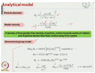
So if you do so we can get an expression for the diameter of the particle, and we can also get an expression for the radial velocity okay. Now if you see this expression, if the density of the particle is larger than the density of the fluid the particle will get subjected to a positive radial force in the outer direction okay, so you know and in for many of the bio-particles that we encounter in microfluidics the density of the particular is greater than the density of the fluid.
