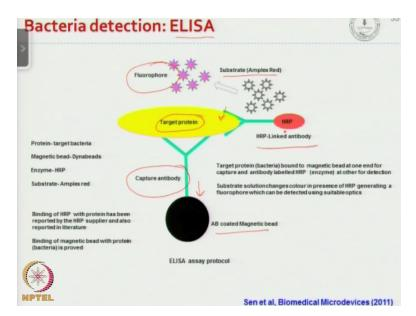
And here we present a microfluidics system that has been developed for detection of bacteria which is based on the ELISA technique which is Enzyme-linked immunosorbent assay okay. So essentially this is the target protein which is the bacteria, and the first we try to capture the bacteria inside the microfluidic device and that is done by capture antibody which is coated onto a magnetic bead, so that capturing is done by this magnetic bead.
