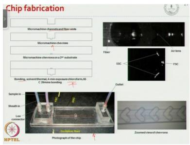
So this is the chip fabrication process, it uses micro-milling and bonding, so it is basically micromachining the channels and the fibers slots, and then micromachining the chevrons at the bottom of the channel, and then a bonding the 2 different wafers using the solvent bonding okay, here chloroform used for the solvent bonding process. So this is an image of the chip that has been fabricated using this method okay, and this is the microflow cytometer chip that we are talking about.
