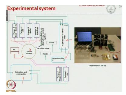
So this is the experimental setup with you know different modules, this is the extraction module so after the extraction and mixing with antibody the bacteria solution is infused to the capture and reaction chip, from there the fluorophore is generated which taken to the detection chip. And all these you know different types of different pumps and valves are actuated using a control system.
