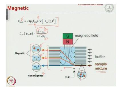
Next, we talk about magnetic based particle separation which also known as magnetophoresis, the magnetophoresis phoretic force is given by this expression. So it is a function of the size of the particle a cube and gradient of the magnetic field square of the magnetic field, and this is the magnetic Clausius-Mossotti factor equivalent to the electrical Clausius-Mossotti factor. So if this is depending on the permeability of the particle as well as the permeability of the medium okay.
