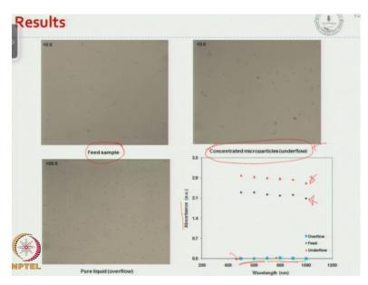
And experiments were performed with particles, so as you can see here this is the feed sample that is put into the device, and this is pure liquid that was collected on the top of the hydrocyclone, and as a result this is the concentrated political that was collected down okay. And also the absorbance measurements were performed, you can see that this is the you know absorbance that is offered by the feed what comes in as the sample.
