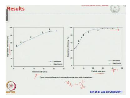
So here we did you know the effect of inlet velocity on the separation efficiency was studied using both simulation and experiment, as you can see that the separation efficiency increases with the inlet velocity. So as the inlet velocity increases the centrifugal force also increases which leads to higher separation efficiency. Here, you can see the increase in the particle size versus separation efficiency.
