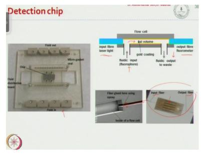
So this is the detection chip that we used to detect the fluorophore based on fluorescence measurement, so essentially we have a flow cell and an inlet and outlet, and the flow cell is interfaced with a input fibre and output fibre. So this is the photograph of the chip that was fabricated and this shows the inside of this flow cell, so this is the flow cell, and here the optical fibers are introduced and the glued around here, this is what you see this is the chip input fibre and output fibre.
