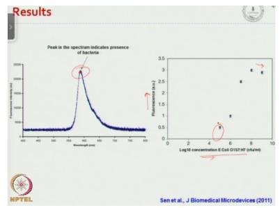
And you know this shows after we put in after we capture and we put in you know the HRP incubate the sample, and then we bring in the substrate solution we have a fluorogenic compound, then that fluorophore is taken into the detector chip, and in the detector chip based on the fluorescence intensity we get a spectrum. So as you can see depending on the intensity we see the fluorescence intensity spectrum we see a peak okay.
