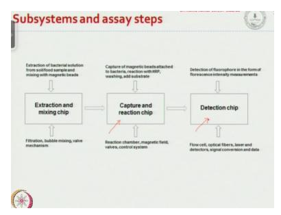
So the system that we talk about has 3 different chips, one is the extraction chip which extract bacteria from soil, and the second chip is the capture chip which captures bacteria inside a microfluidic device, and the third chip is the detection chip which actually detects based on the fluorescence measurement,
