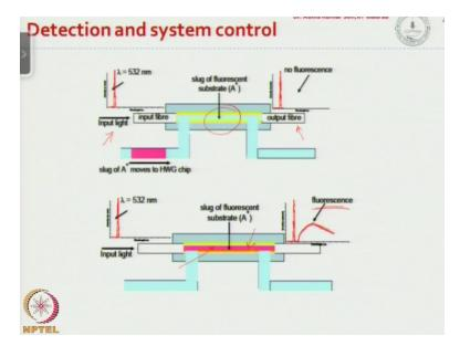
And this is the detection system that is shown here we have the input light that is coming at 532 nanometer, and this is the output light, and here we do not have any fluorogenic fluorophore present, and as the slug of the fluorophore is introduced into the flow cell, we would see a peak in the fluorescence okay. And this fluorescence characterizes the fluorophore here okay.
