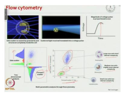
So the forward scatter is caused by the size of the particle, but the side scatter is caused by the internal structure of the particle okay. So when the particle crosses you know the light as you can see here the light signal is collected by what is called a photomultiplier tube and what is known as PMT, and the PMT basically converts the light energy into electrical energy okay. So this electrical energy can be collected using a data acquisition system.
