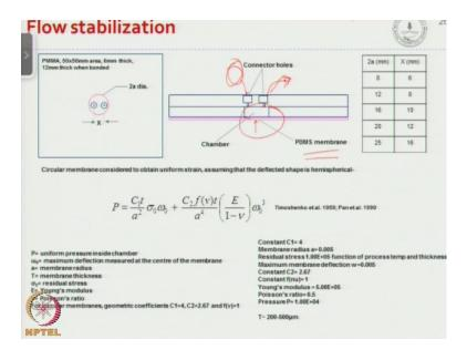
Another mechanism which has been used in this particular micro flow cytometer is a flow stabilizer, as we know that you know to count the particles we need the particle single file, but at the same time this location of the particles need to do not change with respect to the light beam okay, and to achieve that the flows should be very steady, and most of the microfluidic pumps including change pumps are pulsatile in nature.
