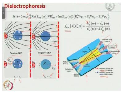
So the first active separation method that we will talk about is dielectrophoresis, the dielectrophoretic force is given by this expression okay 2 pi epsilon m which is the permittivity of the medium\*the cube of the radius and the real part of the Clausius-Mossotti factor okay, and the gradient square of the gradient of the electric field. Now if you look at the Clausius-Mossotti factor it has 2 different components.
