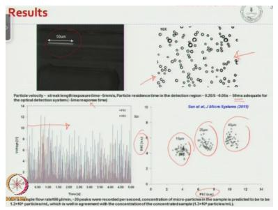
So another important parameter to check here was the residence time of the particle in the detection window, so we could find from the vertical velocity using optical measurements, we could find the residence time is about 50 millisecond which is adequate for the optical detection system that was used which has a response time of about 5 millisecond. Now next, a mixture of particles where put into the microflow cytometer.
