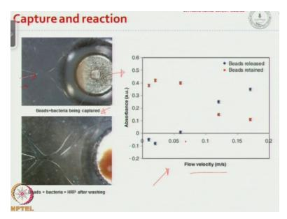
And here we are showing photographs of how the beads and bacteria are being captured using the magnet underneath the chamber, and this is very important study that was made what is the flow rate at which we need to flow the bead bacteria solution for the trapping to occur. If we the flow rate is very high the kinetic energy is more compared to the magnetic energy, then you would have the bead bacteria are getting lost some of them are not getting trapped.
