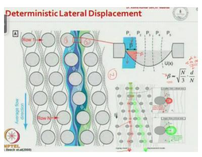
Now if you look at the mechanism between 2 adjacent post, let us say this is post 1 and this is post 2, we have different streamlines okay, so in this case we have 1 2 3 4 streamlines, now if you look at the stream between the surface and the first streamline the width is beta okay. And this beta is expressed as square root of N/3\*d/N, where N is the period of the array, meaning the first and N+1th row have the same configuration okay.
