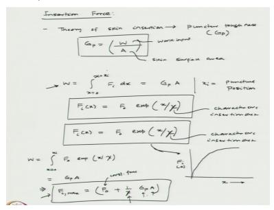
So we look at insertion force the theory of skin insertion is based on the puncture toughness, the puncture toughness of the skin which is expressed as symbol GP, so the puncture toughness can be expressed as the work input the amount of work that we do/the surface area of the skin okay, so this is the work input and this is the skin surface area okay. The total amount of work that we do will vary between x=0.
