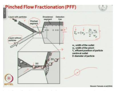
So this is the pinched flow fractionation technique as you can see here, here we have a sample that contains the particles and here we have a buffer which does not have any particle, and this sample is focused by the buffer stream so that the particles get a line to one of the side walls, and this is known as the pinched segment. So this has a lower width of the channel, and as the pure fluid focuses the particulated fluid, the particles get a line to this side wall.
