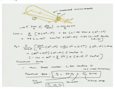
So one such microneedle is shown here, so this is the tapered microneedle, and for the tapered microneedle we can write down E\*I x\*d square/dx square +M x=0, the M x is varying, I x is
