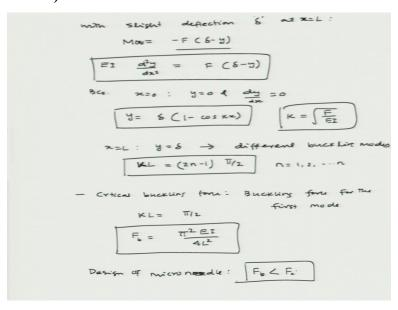
And with a slight reflection delta at x=L which is the end of cantilever, the bending moment M can be written as -F\*delta-y okay at a particular x this can be written as -F\*delta-y, so we can solve this equation d square y/dx square=F\*delta-y. Now to solve this equation what are the boundary conditions we have available, the boundary conditions are x=0 at x=0 that is the clamp and the deflection=0, and also the slope dy/dx is going to be 0.
