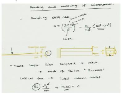
So first let us talk about bending and buckling of microneedles, so the bending stiffness of a needle so let us call it K which is given by okay 3 E I/L cube okay, so basically this is a cantilever type of structure the microneedle becomes like a cantilever type of structure, and this is the buckling force which is applied here. And this leads to deflection of the cantilever okay, so if the length is L, and I is the moment of inertia.
