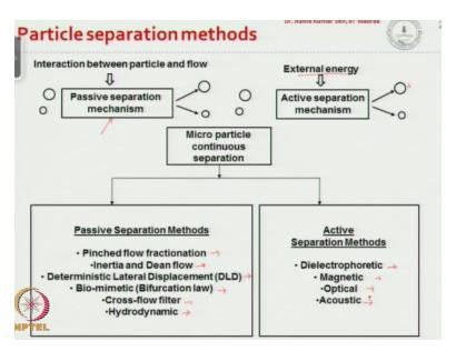
So we talked about microparticle separation, microparticle separation as different applications in biomedical and in chemical analysis, it also has applications in chemical industry, mineral industry and the many other applications that it sees okay. So let us look at the principle of different principles of microparticle separation. So as you can see here the microparticle separation is broadly classified into 2 categories, one is the passive separation.
