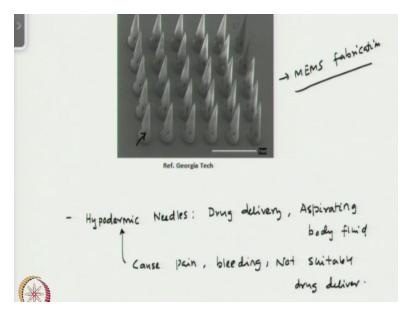
Now if we so here we look at one example of microneedles which has been developed at Georgia Tech, so these microneedles have been fabricated using MEMS fabrication okay, and as you can see these are pointed structures which can pierce into the skin and the there are some openings as you can see here which through which the drug can come out okay. So first let us look at why we use microneedles?
