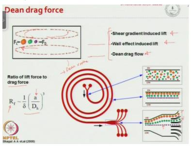
Next, we move onto a dean drag force, so the dean drag force mechanism is based on 3 different kind of forces, here as you can see we have shear gradient induced lift, we have wall induced lift and dean drag flow okay. Now when particles move inside a fluid in a channel the difference you know if a particle is moving through a channel the difference between the particle velocity and the liquid velocity is higher closer to the channel as compared to that of particle closer to the center okay.
