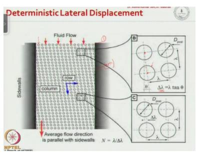
Next, we look at a technique all deterministic lateral displacement or DLD, here we have in the channel an array of post that are sticking from the channel okay, and the deterministic lateral displacement is based on the principle of steric hindrance. Steric hindrance means the wall is trying to apply force on the particle to escape from one streamline to get into another streamline okay that is known as steric hindrance okay.
