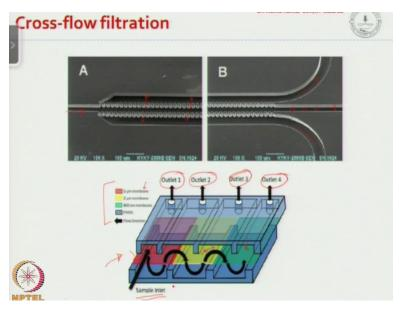
So next we move onto cross-flow filtration, in cross-flow filtration you know we have so as you can see here let us say the particles sample comes in here. And you know the difference between the cross-flow filter and the dead and filter is that, in cross-flow filter the filtration occurs in a direction perpendicular to the normal to the flow direction okay, so that is how the pores of the filter do not get clogged and continuous filtration is possible.
