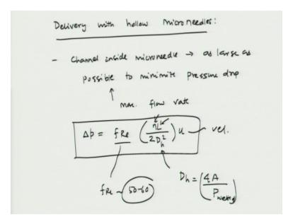
So now let us look at the flow characteristics of a micro needle, so look at the delivery with hollow microneedles, so you know one of our goals while designing microneedles from the perspective of flow is that the pressure drop has to be small as possible okay, and for that we need the inner bore of the microneedle has to be as large as possible to reduce back pressure okay. So we need the channel inside microneedle as large as possible to minimize pressure drop okay.
