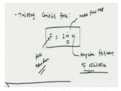
So, in that case we would have a twisting Coriolis force that acts on the tube and that Coriolis illness F is given by 2 \* m dot \* omega, okay. So, m dot is the mass flow rate and the Omega is the angular frequency of oscillation, okay. So, by measuring this twisting Coriolis force which can be measured, using a force transducer. We will be able to predict m dot knowing the angular frequency of oscillation.
