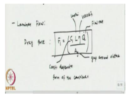
And by measuring the drag, you can predict what is going to be the flow rate. Let us say, and that obstacle could be; for example, cantilever, okay. Now, if you assume laminar flow, let us say we are talking about laminar flow, which is often the case in micro channel, then the drag force will be experienced all in the direction of the flow, okay. So, the drag force is going to be F1 will be C1 \* L Eta Q dot/ Ag.
