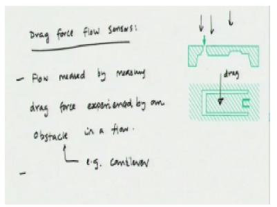
Now, let us look at drag force flow sensors. So, let us look at drag force flow sensors; the drag force flow sensors work on the principle that we would introduce an obstruction like a cantilever structure into the flow field and when the flow rate would change, the drag experienced by the cantilever is going to change okay and by measuring the drag; change in the drag can be used to predict the flow rate.
