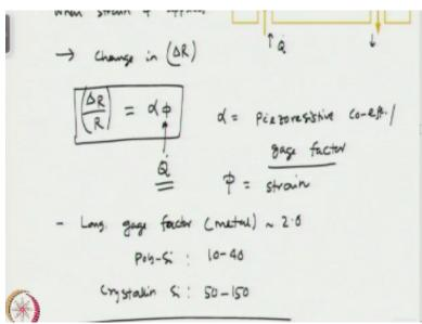
And because the change in the pressure, there is a deflection of the member for which the resistance r between the 2 electrodes, which is a function of flow rate, okay. So, when the strain phi is applied, so we would have change in electrical resistance, okay. So, change in resistance, so delta; so this delta R over R is going to be a function of strain. So, let us alpha \* phi and this alpha is the piezo resistive coefficient or for the strain gage, it is the gage factor.
