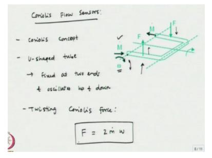
So, that is the principle of operation of the lift force flow sensor. Now, let us look at Coriolis flow sensors. So, let us look at the Coriolis flow sensors; so, the Coriolis flow sensors are based on the principle of Coriolis concept, okay. So, as you can see here, this is the U shaped bent tube, okay and the flow is getting in there, so this is the must flow rate sensor; some mass flow rate M dot is going inside the tube and coming out there, right.
