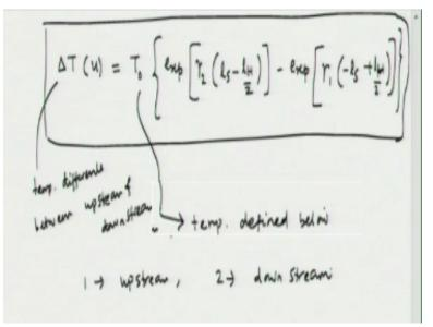
And we would have 2 temperature sensors to measure upstream and downstream temperatures, so that would give us flow rate, okay. So, the difference in the temperature between upstream and downstream; delta T as a function of the velocity has been estimated as T0 \* exponential gamma 2 \* ls - lH/2 - exponential, gamma 1 \* - ls + lH/2, okay. So, this is the expression for the temperature difference between the upstream and downstream.
