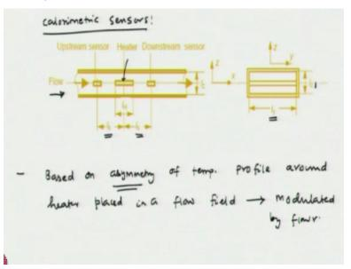
So, by knowing the heating power, we can calculate Nusselt number and from the Nusselt number will be able to calculate the flow velocity, so you can predict what is going to be the flow rate, okay. So, that is how the hot wire sensors work. Now, let us look at calorimetric sensors. So, the calorimetric sensors work on the principle that if you have a hot surface and the hot body and
