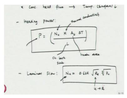
So, the heating power p Nusselt number \* conductivity \* area of the heater delta T/ L, okay. So, this is the Nusselt number, this is thermal conductivity and this is the characteristic length scale, okay, this is the heater area, delta T is the temperature difference and for laminar flow, we have an expression for Nusselt number, which is square root of Re \* Prandatl number to the power 1/3, okay.
