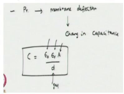
So, membrane itself as one electrode, the counter electrode which is typically fixed and what happens is the pressure causes the membrane deflection, okay; pressure causes the membrane to deflect and the membrane deflection will cause change in the capacitance, okay. So, we can write down the expression for capacitance which is epsilon 0, epsilon r, A/d, so this is permittivity of free space.
