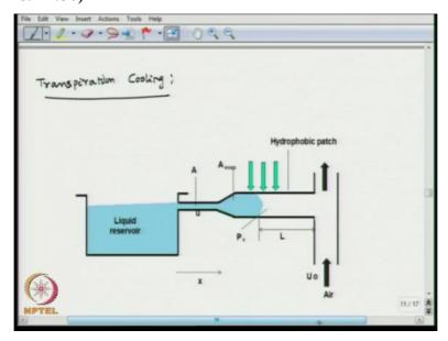
So, similar effect that is discussed here, so we have a liquid reservoir in which liquid is present and so by capillary action, the liquid is allowed to go through this capillary until a point where we have a hydrophobic patch, so this area of capillary has got a hydrophobic
