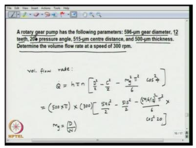
So this is the very simple question, if you remember the formula. The volume flow rate for a gear pump is given by h\*pi n d square/2 - c square/2 - mg square pi square over 6\*cosine phi square, okay. So this is the expression for the flow rate for the gear pump, so h is the channel height, so it is given which is 500 micron\*pi\*n is the rpm which is 300\*d square by 2 is 596 square by 2 - the center to center distance is 515 square by 2.
