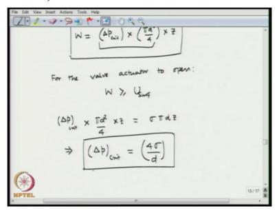
So, we get the surface energy as sigma\*pi d\*z, right. Now, the external force will be applied, okay so this would cause mechanical valve. So, the external force applied has to overcome the critical pressure that is required to open the valve, okay. So, the external force, so total worked on would be delta P critical that is the critical pressure to open the valve\*the area which is pi d square over 4\*so that force is applied over a distance z, okay.
