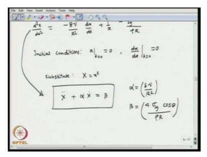
This term is going to be negligible, okay. So this term is going to be negligible, so we can simplify the equation for this term vanishes, so d square x over d t square = - 8 nu over R square dx over dt + 1 over x 2 sigma lg cosine theta over rho R, okay. Now, we can write the initial conditions, the initial conditions are x at t = 0 is going to be 0 and dx over dt at t = 0 is going to be 0.
