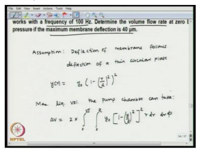
So, the deflection of membrane follows deflection of a thin circular plate, so in that case we can write the deflection y r as y0 1- r over R square whole square. So, we can find the maximum volume that the pump chamber can take, the maximum liquid volume the pump chamber can take which is given by delta v will be twice 0 to 2 pi\*0 to R y0\*1 - y over R square whole square r dr\*dr\*phi.
