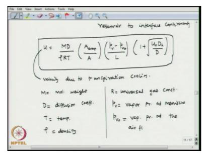
So this is the expression for the velocity due to transpiration cooling, okay. So, U is the velocity due to transpiration cooling, M is the molecular weight and D is the diffusion coefficient, T is the temperature and rho is the density, R is the universal gas constant and Pv is the vapor pressure at the meniscus and Pv0 is the vapor pressure at the air flow side, okay. The area of the evaporator and the area of the cross-section of the channel are given.
