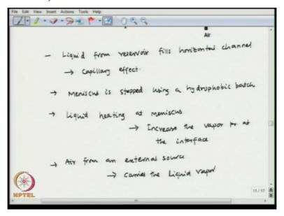
So, we would have air from an external source, the air will carry the liquid vapor and that would create a vapor pressure gradient, that would create a gradient of pressure, okay. So that will enable the liquid to come in continuously to the interface. So, liquid comes in from reservoir through interface continuously, okay and that velocity is given by this expression, M\*D over rho R T and\*A\*evaporator over A Pv - Pv0 divided by L\*1 + U0 Dh over D.
