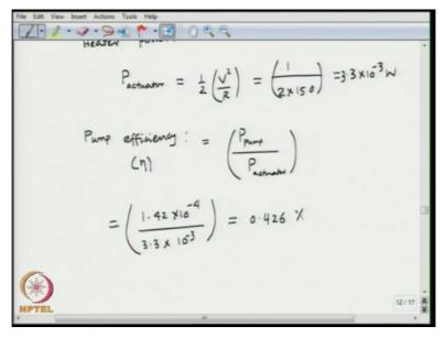
We can find the power of the pump as P max, so this is pump of P max Q max divided by 2, so that will be P max is 50 kilopascal, 50\*10 to the power 3 and Q max is 340 microliter per minute, so 340\*10 to the power -9 divided by 60 meter cube per second divided by 2, so that would be 1.42\*10 to the power -4 watt, okay. Similarly, you can find heater power, okay.
