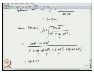
So first, we have to calculate what is the burst frequency when at the distance where the liquid column is located 4 millimeter, then we can calculate what will be burst frequency when it will be located at 16 millimeter, okay. So, the first thing to do is calculate the hydraulic dia, the hydraulic diameter can be calculated as Dh is 4\*area of cross-section over perimeter.
