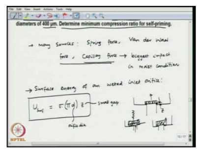
Now, for a check valve pump, there are many sources to hold the valve in place, we have the spring force or we can have thermopneumatic force which can hold it in place, okay. So, we will have many sources like spring force or Van der Waals force or we can have capillary force, okay. So, these are different sources that can be used to close a valve. Now, for a valve that is handling liquid since the condition is moist, the capillary force based valve closing is more significant, okay.
