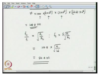
So what is going to be at 16 millimeter, we can find f2 or 16 millimeter is going to be f1\*R1 over R2 square root, so this will be equal to 108.8\*4 over 16 square, so that will be 54.4 hertz, okay, right; So with that, let us stop here.
