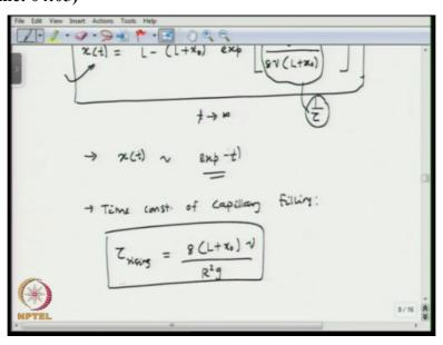
So, we can define a time constant for the filling process which will be given by this expression. So this is the time constant, this actually inverse of t, 1 over tau, we can define a time constant of capillary filling, okay. So, tau rising 8\*L + x0 nu divided by R square g, okay. So, the time constant is an indicator of how much time is going to take for the capillary rise to occur.
