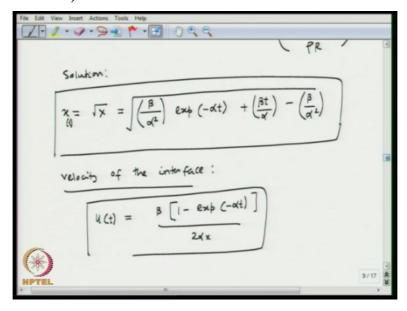
So, the solution would be x will be square root of X which is beta over alpha square\*exponential - alpha t + beta t over alpha - beta over alpha square, okay square root. So that is how x is going to vary with time, okay. So, x is function of time, from there, we can obtain an expression for the velocity, okay. So, the velocity of the interface u is a function of t is going to be beta.
