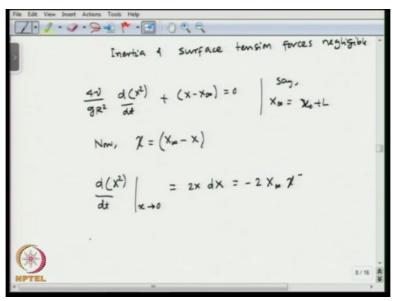
So in the general equation, if you drop of the inertia and surface tension forces, then we get 4 nu over g R square\*d of x square over dt + x - x infinity are 0, where we say that x infinity is x0 + L, okay. So, now if you consider a parameter x as x infinity - X, we can say that d x square over dt at x tends to 0 will be 2x\*dx this will be = - 2 x infinity\*x. So, this is what we can say.
