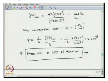
So, 400\*10 to the power -6, so that is going to be 720 Pascal. So, we need minimum 720 Pascal to open the valve, okay. So, we can find the minimum compression ratio, the minimum compression ratio which is psi which is nothing but delta v over v0, right. So, we have an expression for psi for liquid, so that is going to be 1 over K\*delta P critical divided by P0. So, this is something that we have seen in the previous lecture.
