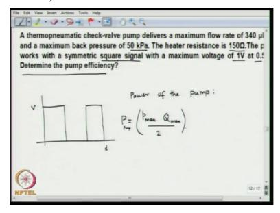
The pump works with a symmetric square signal with a maximum voltage of 1 volt at 0.5 hertz and we want to determine the pump efficiency, okay. So, how do we do that? So first, you know we would have this is time and this is voltage, so we have a power signal that is being applied. So this is applied for only one half of the cycle, okay. So, we can find out the power of the pump.
