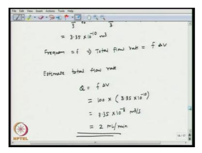
So, we get 2 pi over 3\*y0 R square that will be 2 pi over 3, the maximum deflection is given as 40 micron, so this will be 4\*10 to the power -5\*the radius of the membrane is given, so it is 4 millimeter diameter, so the radius is 2 millimeter, 2\*10 to the power -3 square, so that will be 3.35\*10 to the power -10 meter cube. So this is going to be the liquid volume, the pump chamber can take in a single stroke.
