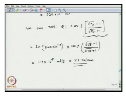
So, let us consider another example, so this is the rotary gear pump that we have discussed and it has the following parameter, it has 596 micron of gear diameter and it has 12 number of teeth and the pressure angle is 20 degrees, okay. So, 20 degrees pressure angle and 515 micron center to center distance, okay and the thickness is 500 micron which is equal to the channel height and we are going to determine the volume flow rate a speed of 300 micron.
