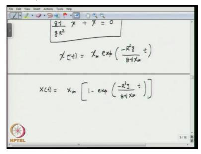
Now, we can convert it back to the small x t which is our original variable, x t is going to be L - L + x0 exponential - R square g divided by 8 nu\*L + x0\*t, okay. So that is the solution we would have at the end of the filling process when t tends to infinity, okay. So, what we see here is that the profile is going to reach a steady state exponential, okay. So, x t varies as exponential t, okay.
