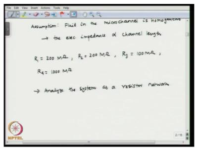
Because the total is 400 mega-Ohm, so R2 will be 200 mega-Ohm and R3 will be 100 mega-Ohm and R4 will be 1000 mega-Ohm. So R3 has half the channel length, okay. So R3 is only 10 millimeter, so it will be half of R12 junction, okay so that is 100 mega-Ohm and R4 is 10 times R3 so that will be 1000 mega-Ohm. So, we can analyze the system as a resistor ne2rk.
