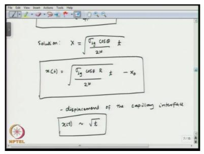
So, the inertia and the gravitational force are going to be negligible, so this is the general equation we work on and for the beginning process, we drop the inertia and the gravitational force from this equation and if we do that we get this simple equation, we get 8 mu over R square rho\*dx over dt - 2 sigma lg cosine theta over rho R\*1 over x + x0 is going to be 0. So, we can do a conversion of a variable, we can say X is x + x0, okay.
