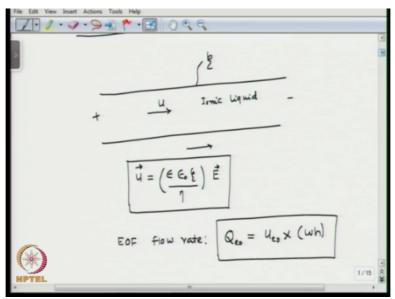
So, we talk about electrokinetic micropump, so here we have a channel which has some zeta potential, okay and here inside we have an ionic liquid, liquid with non0 conductivity and if we establish an electric field, okay then we induce a electro-osmotic flow, okay and this electro-osmotic flow velocity is given by epsilon epsilon 0, so that is the permittivity of free space, this is a dielectric constant of the liquid\*zeta potential over the viscosity of the liquid\*the electric field, okay.
