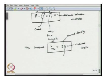
So, you can find out the expression for the pressure and flow, so the maximum pressure P max has been estimated as J\*B\*L, okay. So, J is the current density, okay and B is the magnetic flux intensity which is defined here and L is the channel length, okay and the maximum flow rate Q can be defined as J\*B\*pi Dh4 divided by 128, okay. So that is the expression for the flow rate.
