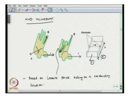
So, if you have a channel such that you are applying a current in the thumb direction and you are applying a magnetic field along the index finger, the liquid will be subjected to a force along the middle finger, okay. So that is the principle based on which the magneto-hydrodynamic pumping works. So as we can see here, so this is the direction of the current and this is the direction of the magnetic field.
