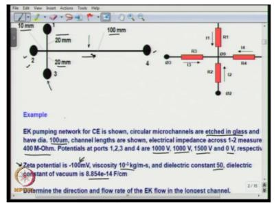
So that is the principle of capillary electrophoresis. Here one such ne2rk is shown and we have circular microchannel cross-section that are etched in glass and have diameter of 100 micron and how do you make circular microchannels? We can have bulk etching of silicon to have hemispherical channel and we can bond 2 such microchannel to get a circular microchannel cross-section and here all the channel lengths are shown.
