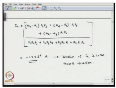
So that will be same as the direction of the flow, okay. So, what that means is direction of I4 is in the reverse direction. So, it is going from the junction towards the port 4, is in the reverse direction. Now, you can find the electric field strength in the longest channel, which is going to be phi0, phi0 is the potential at the center - phi4 divided by L. So, this is going to be I4R4 divided by L.
