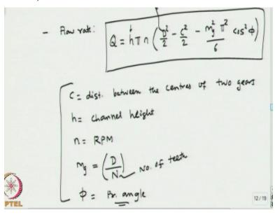
So, flow rate has been estimated we can express in terms of a formula h pi\*n\*d square/2-c square/2-mg2 pi square/6\*cos square pi. So, this is the expression for the flow rate here you can see D is the diameter of the gear okay and so this is the gear dia and c is the distance between the centers of the 2 gears. So, c is the distance between the centers of 2 gears and h is the channel
