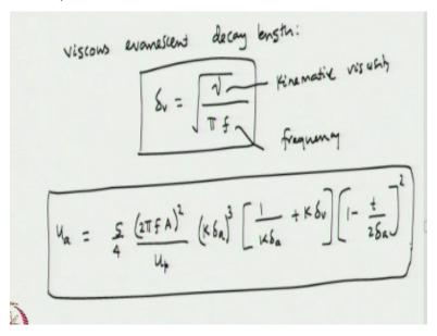
And then you have the viscous evanescent decay length viscous evanescent decay length which is given by the expression nu/pi\*f square root okay so here nu is the kinematic viscosity and the kinematic viscosity and f is the frequency of the acoustic wave okay. Now the acoustic streaming velocity ua can be determined this ua can be determined as so this is the velocity of the liquid okay.
