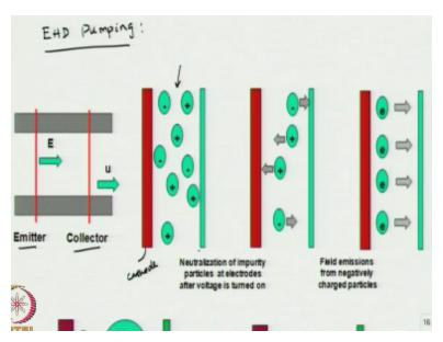
So, we look at EHD electro hydro dynamic pumping which is different than electro kinetic pumping normally in electric kinetic pumping we use relatively low voltage is as compared to what to use in electro hydro dynamic pumping okay. So this is the typical configuration of an electro hydro dynamic pump. So, there will be pairs of emitters and collectors so initially the liquid that is present between the emitter and collector may have some impurities okay.
