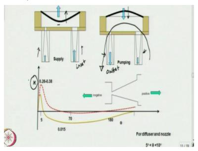
So this is a configuration of a valve less micro pump that you see here and what happens is when the membrane is trying to move up as you can see here then it creates a negative pressure inside the chamber and so during that time. So, this is the inlet it okay so this is the inlet and that is the outlet so when the negative pressure is created here the liquids move from the inlet into the chamber also some liquid move from the outlet into the chamber.
