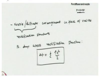
So, here we use nozzle diffuser arrangement in valve less micro pump we use nozzle diffuser arrangement and instead of in place of valves okay. So, the pressure loss across nozzle diffuser that is called rectification structure. So, these are called rectification structures okay so that means the flow has a directionality depending on the pressure drop nozzle diffuser okay. So, the pressure drop across the rectification structure.
