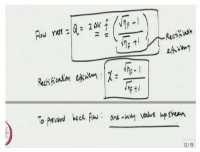
So, we can write an expression for the flow rate can be written as Q is 2\*delta v\*f f is the frequency of the oscillation of the membrane\*square root of etaf-1/square root of etaf+1, eta f is the fluidic diodicity So, that is how we can express the flow rate given by a valve less micro pump in terms of the stroke volume and the frequency and the diodicity. Now this parameter here is known as the rectification efficiency okay.
