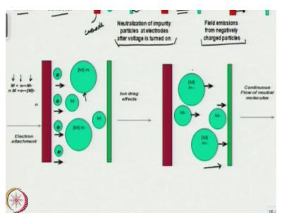
And these electrons are going to interact with the molecules of the liquid okay and make it negatively charged you can see here the electron is interacting with this molecule to make it negatively charged and so now these molecules become negative charged and so they will migrate towards anode so they migrate towards anode in doing so they carry the bulk of the liquid with them okay.
