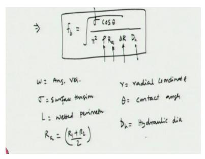
Dh is the hydraulic diameter of the channel okay say Dh is the hydraulic diameter of the channel then from here we can predict what is going to be the burst frequency ok fb is going to be sigma cos theta/pi square rho Ra\*delta r\*Dh square. So, the burst frequency depends on the surface tension of the liquid channel interface and it depends on the contact angle it is inversely proportional to the density.
