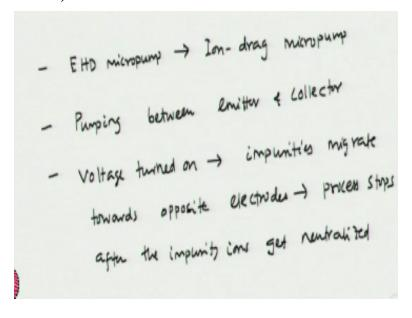
So, here in this case we also call the EHD micro pump we call it as iron drag micro pump here we have a pumping between emitter and collector pair of electrodes and initially there may be some impurity present when voltage is turned on the impurities migrate towards opposite electrodes ok and this is going to be a short process and that they stop as soon as the charge just neutralized okay.
