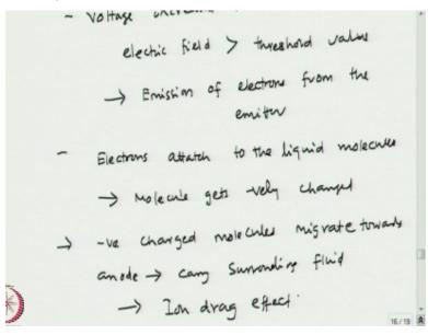
And if you have voltage increased further then and the electric field L is greater than the threshold value then you have emission of electrons from the emitter okay and these electrons would attach to the molecules attach to the liquid molecules. And so the molecules get a negative charge okay and these negative charge molecules migrate towards anode. So, they carry surrounding fluid which is called ion drag micro pump.
