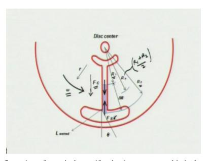
So this is the configuration of a typical centrifugal micro pump so this is the disc center about which the disc is rotated at under velocity of omega and this is the liquid column that we are trying to analyze here. So, this liquid column the bottom end is at a radius of R1 the leading edge is at a radius of R2 and the average radius R1+R2/2 is RA, so this is R1+R2/2. So for this liquid column.
