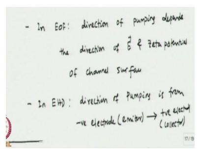
So, we can say here in electroosmotic flow the EOF flow the direction of pumping depends on the direction of the electric field. And the zeta potential of channel surface whereas in HD pumping the direction of pumping is from the negative electrode is also known as the emitter towards the positive electrode and collector okay. So, that discussion we will move on and talk about electro kinetic micro pump.
