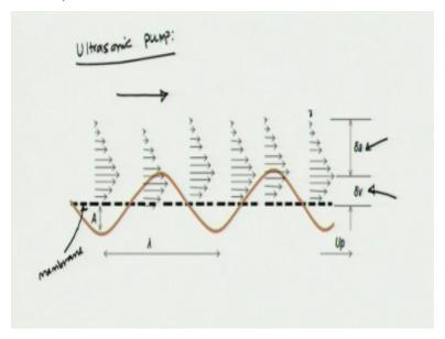
So, this is the ultrasonic pump okay so here we have a this is the membrane we are talking about this is the thin membrane coated with the electrodes okay and when you know the electrodes are excited the membrane will undergo oscillation. Okay so these mechanical waves will be traveling on the surface of the membrane okay. So, when the mechanical waves will travel on the surface of the membrane.
