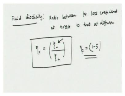
So, we can define the parameters which is called the fluid diodicity which is the ratio between pressure loss coefficients at nozzle to that at diffuser okay. So, we defined fluid diodicity we defined where the parameter eta f which is given by xi- pressure less coefficient for the nozzle/pressure loss coefficient for the diffuser okay. So, eta f has a value typically between 1 to 5 okay.
