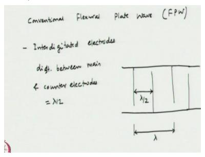
Normally we use okay in a conventional flexural plate wave is FPW flexural plate where we have interdigitated electrodes okay. So, on the surface of this membrane we would have interdigitated electrodes that will cause the acoustic waves and let us say in a configuration we have the distance between we have a configuration something like this okay so let us say this is the separation distance between the main and counter lambda and between 2 electrodes lambda/2.
