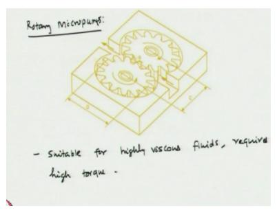
So, we talk about rotary micro pumps so rotary micro pumps have 2 gears which are driven in opposite to each other to drive very viscous fluids okay. So, rotary micro pumps are used for driving viscous fluids and so it requires high torque is necessary. Okay the rotary micro pumps are suitable for highly viscous fluid and so it requires high torque so we need external actuator and the flow rate of such rotary pumps have been estimated.
