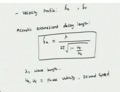
Okay so the velocity profile is characterized by 2 parameters the velocity profile characterized by the acoustic evanescent length and the viscous evanescent length. The acoustic evanescent length acoustic evanescent dk length which is delta a is given by the expression lambda/2 pi square root of 1-up/ub, so here lambda is the wave length okay. So, when you have this flexural wave this is
