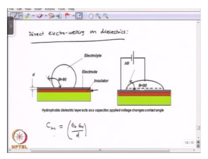
So we talk about direct electrowetting on dielectrics. So as you see here instead of having the electric layer we add one more insulating layer here, so we have the capacitance of this insulating layer plus the capacitance of the electrical double layer. So the capacitance of the insulating layer, which can be controlled is given by epsilon 0 epsilon r/d okay.
