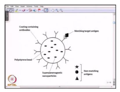
So you know here we see an example so this is the polystyrene bead okay and which is not magnetic and here this polystyrene bead is made magnetic by having these super paramagnetic nanoparticles inside okay. The super paramagnetic means you know these particles will go back to their non-magnetic nature when the magnetic field is taken out that is called superparamagnetic okay.
