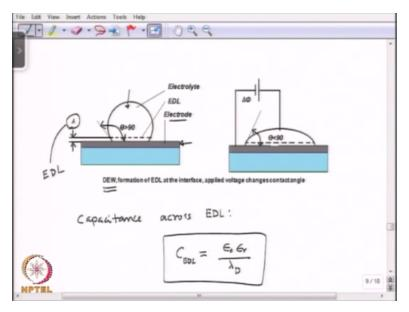
So as you see here we have a solid electrode okay, this is the electrode and we have an electrolyte okay. So in this case we can expect direct electrowetting at the interface between the electrically conducting liquid and the solid electrode. We would have an electrical double layer that would exist okay because the liquid has non-zero conductivity. So we would have an electrical this is the electrical double layer okay.
