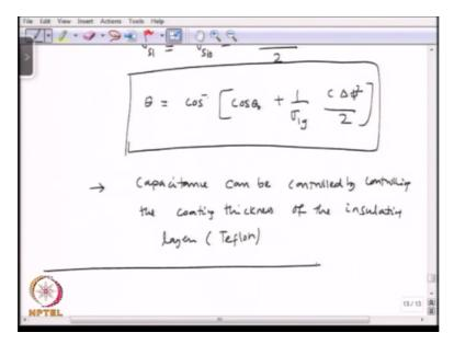
So here the capacitance can be controlled by controlling the coating thickness of the insulating layer which could be for example Teflon okay. So with that let us stop here.
