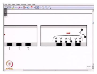
So this is 1 such case shown here. What we see here? This is a microchannel okay so this is the width of the microchannel and we have these magnets present these 3 black rectangles that we see is there you know magnets and we flow these magnetic bead attached to antibody okay what do we see here is this is the magnetic bead attached to the antibody, which is specific to a particular antigen through the microchannel.
