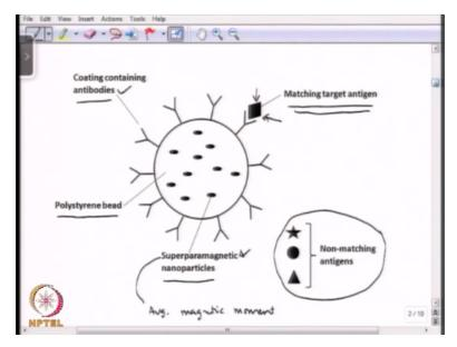
So they are present inside this polystyrene bead so the bead acts as a magnetic particle okay. On the bead, we have a coating of antibodies okay and you know in a sample we may have various different types of antigens and only the matching target antigen will bind to these antibodies okay so these are the antibodies coated onto this magnetic bead and only the matching target antigen will be bound to these antibodies.
