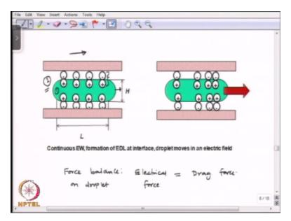
So you can see this here. We are talking about the interface between 2 electrical conductive liquids so you have 1 liquid here which is in the form of droplet and this is the other liquid that we are talking about which is the continuous phase and because of non-zero conductivity at the interface, we would have an electrical double layer that would exist and if we apply an electric field okay.
