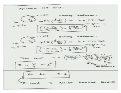
So we consider dynamic heat transfer case, here we have a hot body let us say initially at temperature Ti and in an ambient at T infinity, so Ti>T infinity, and the temperature of it is going to vary as T with time okay, so we can write you know the energy balance we can write rho density of the object\*C specific heat-dT/dt because the temperature is going to reduce with the time, so there is a negative sign here is going to be h A\*T-T infinity.
