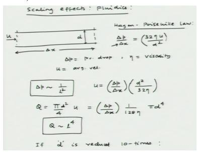
So we talk about scaling effects in fluidics, so here we consider a straight channel of diameter d let us say this d and the velocity is u, let us say delta x is the length of the channel okay, so you know we know that in case of laminar flow through a channel or a tube we can apply the Hagen–Poiseuille law, so if you apply the Hagen–Poiseuille law, we can write delta p/delta x is going to be 32 eta u/d square.
