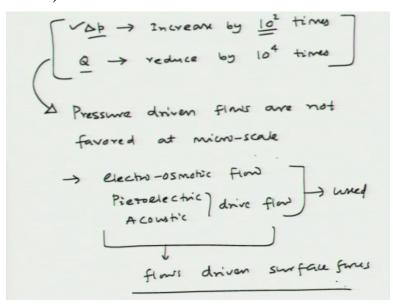
On the other hand, the Q is going to reduce by 10 to the power 2 times okay right, this is 10 to the power 2 times because pressure scales as 1 square right delta p scales as 1 square, so you are going to reduce 100 times as 1 is reduced 10 times, then Q delta p is going to increase by 100 times when d is reduced 10 times, and the flow rate is going to reduce by 10 to the power 4 times, so both effects are undesirable effects.
