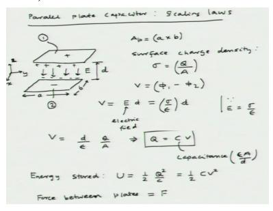
So we are going to look at parallel plate actuator capacitor, and we will look at how the scaling law is going to work? Okay, so you know we can draw 2 parallel plates here this is one plate and this is another plate, let us consider this is y, this is x sorry this is z and this is x, and we say this is plate 1, and this is plate 2, this is negatively charged plate so we have negative charges here, this positive okay. So the electric field is going to be in this direction E.
