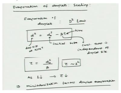
Now let us look at another microsystem, how you know the evaporation of the droplet is going to scale with the length scale okay. So we look at evaporation of droplets how the scaling is going to work, so we know that the evaporation of the droplets is going to follow what is called D Square Law okay, so evaporation of droplet going to use D Square Law okay, what it means is that d square=d0 square-beta t okay.
