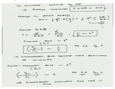
So the force between the plates let us call it F, and to increase spacing by delta Z, the energy required would be F\*delta Z, so let us call this delta W as the energy required. Now the corresponding change in the energy stored, so change in stored energy we can find delta U will be 1/2 Q square\*change in the capacitance, because the total charge is going to remain unchanged, so the moving the plates would change the capacitance.
