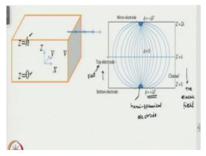
So, this is the case we have here; you know we are talking about a rectangular channel, so you know the bottom wall is at z = 0 and the top wall is at z = h, so you know the flow is in the x direction; the positive x direction. So, what we have here; you know as I told for the dielectrophoretic action to come into play, there has to be a non-uniform electric field okay, so if you look at here, you know we have an asymmetric electrode configuration.
