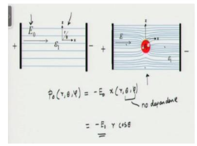
And we would see how the dielectric moment; you know the dipole moment is going to vary in space okay. So, this is the situation will be talking about, so here we have a positively charged plate and negatively charged plate, so we establish an electric field okay and let us say the dielectric constant of the fluid is epsilon 1 okay, so you know that the dielectric fluid here is being penetrated by the electric field epsilon 0.
