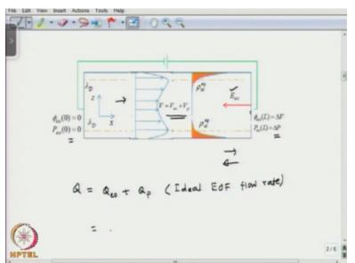
You know, this is the situation we have been looking at. We have been looking at flow in a circular pipe where we have the walls positive zeta potential and the electric field is in this direction as you can see here. So, we would expect the electroosmotic flow to occur from left to right okay in this direction and that the pressure gradient is positive in this direction. We have delta P and P=0 here. So, the pressure driven flow is going to occur from right to left, okay.
