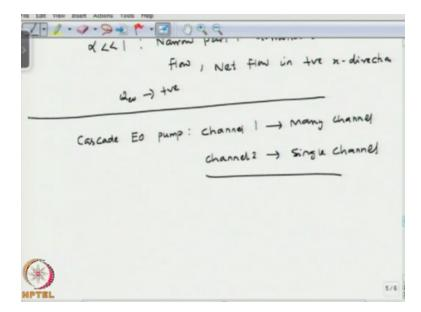
So, that is called the mini cascade electroosmotic pump where we would have the channel 1 was many channel and channel 2 was single channel, okay.
