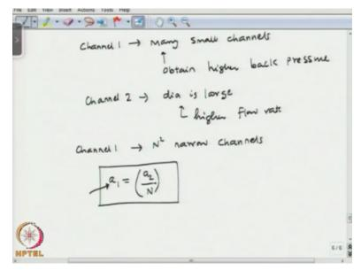
So, the idea is the channel 1 is divided into many small channels and that is to obtain higher backpressure, okay and the channel 2 the dia is large to obtain higher flow rate, okay. So, let us say we have divided the part 1 into n square channels. There are n square different parallel channels here, okay. So, channel 1 has n square narrow channels. So, we say that a1=a2/N. So, the size of the channel in part 1 is a 1/N\*the size of the channel in part 2, okay.
