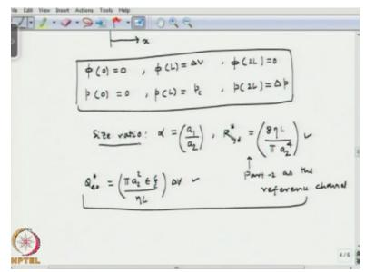
So, you know we see that the phi at x=0 is 0 and we can see pressure 0=0 is 0 and the phi at x=L is going to be delta V and P at x=L is some Pc, okay and phi at x=2L is going to be 0 and pressure at x=2L=delta p. So, these are the boundary conditions and we apply that to this situation here where we have 2 channels in series and we have the potential difference as shown here, okay.
