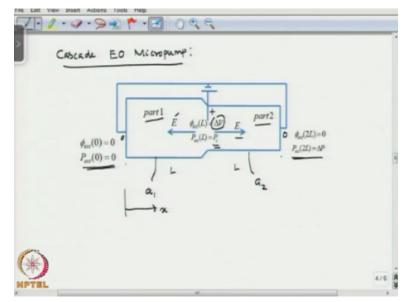
So, what we see here is a cascade electroosmotic micropump, so we call it cascade electroosmotic micropump, okay. So, we have a section of the channel, okay part 1 and part 2. Part 1 has channel size a1 and part 2 has channel size a2 and we have the positive terminal at the intersection between 2 parts somewhere in the middle here, so this is positive and the other 2, this here the potential is 0 and here the potential is 0 and the potential here is some delta v, okay.
