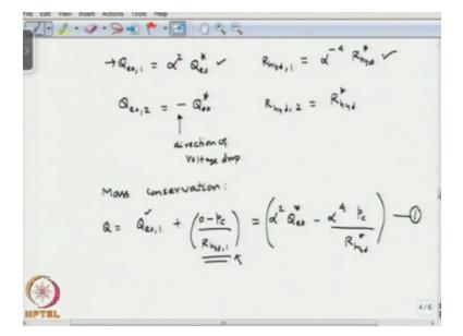
Knowing the size ratio alpha, we can write the electroosmotic flow rate in part 1 of the channel is going to be alpha square\*Qeo star, okay. Similarly, you can check Qeo2 and this is going to be – Qeo star. This negative sign here is because of the direction of the voltage drop. So, as I told the zeta potential is positive. So, the electroosmotic flow occurs in the direction opposite to that of the electric field.
