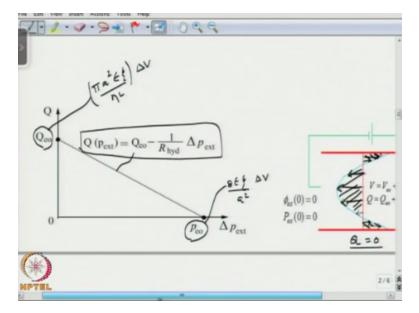
So, here we see the PQ characteristics plotted, okay. This is Peo which is given by 8epsilon xi/a square\*delta v and this is the maximum flow rate which is given by pia square epsilon xi over eta L\*delta v, okay. So, this is the maximum flow rate when the pressure is 0 and this is the maximum pressure when flow is 0, okay and the curve is given by this equation here. What do you mean by when Q is 0 when you get maximum pressure, what we mean is this, okay?
