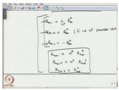
Now, we can define the hydraulic resistances Qeo1=1/N square\*Qeo star and QeoN for n different channels is going to be Q, okay. So, the subscript N refers to N square parallel channels, okay and Qeo2 is going to be –Qeo star, okay. Similarly, we can obtain the expression for the hydraulic resistance, R hydraulic 1 is going to be N4\*R hydraulic star and R hydraulic N is going to be N square R hydraulic star and R hydraulic 2 is going to be R hydraulic star, okay.
