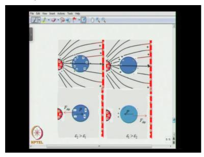
So dielectrophoresis is the force exerted on dielectric or neutral particles subjected to non uniform electric field okay. So one application of dielectrophoresis would be to separate neutral objects like cells based on their physical properties. Dielectrophoresis as I said is the movement of these neutral objects or dielectric objects when they are subjected to a non uniform electric field okay.
