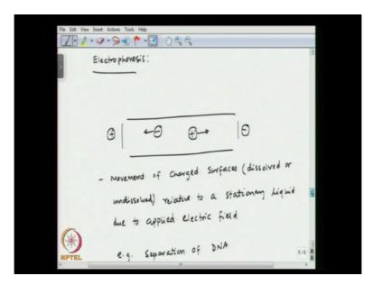
So, we talk about electrophoresis, here we have a capillary or a channel, which has some charge particles let us say negative charge, positive charge and we have electrodes, let us say this is anode and this is cathode. So when we apply this electric field, the charges will migrate towards opposite electrode okay. So because of that, these charges would get separated. So, the definition of electrophoresis would be movement of charged surfaces.
