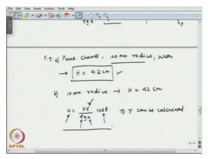
So, now if you take an example, so you consider one example, let us consider a PMMA channel and let us say 100 micron radius you can find that the capillary height is going to be 4.2 centimeter, okay and if you consider water as the liquid. So, you know the density H is going to be 4.2 centimeter. Now if you instead of 100 micron radius, okay if you go for the same material and the liquid water and the radius is 10 micron then H will be 10 times, okay.
