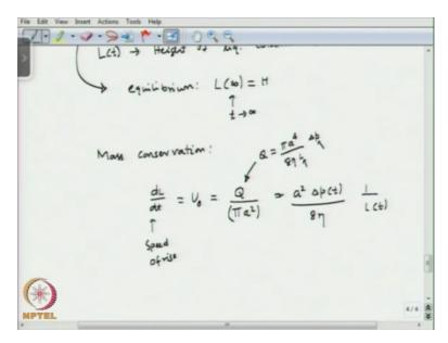
So, next we move on to talk about the capillary rise time, okay. So, we know that if you put a capillary or a micro channel we can expose to some liquid because of the capillary action the liquid will move into, okay. And we found an expression for in case of a vertical capillary what is going to be the maximum height to which liquid will move.
