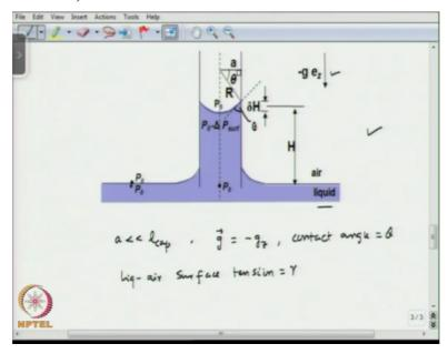
So let us look at, move on to here, so this is the illustrative figure. So, you look at capillary rise height. So, this is the situation as you have see here, okay. For simplicity we are considering a vertical tube into a liquid present here and we are satisfying the condition that the radius of the capillary is << the characteristic capillary length and the gravity is in the vertical direction, okay.
