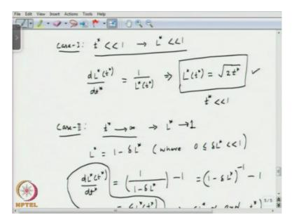
So, use some characteristic scales, we can say t is the characteristic capillary time scale\*t star and where zeta capillary will be = 8 eta H over rho g a square and we can say L will be = H\*L star, okay. H is the maximum capillary height and L is at time t. Now with that we can write this equation in non-dimensional form, so you can write d L star t star of d t star. So, d L t over d L start t star of d t star = 1 divided by L star t star - 1.
