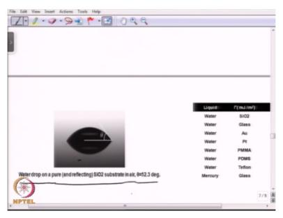
If you look at here, this is the case where the water drop is present on a pure silicon dioxide substrate in air, okay. So, this is silicon water drop present on silicon dioxide surface and the contact angle is about 52.3 degrees which is the theta that is shown here. Now if you want to derive an expression for contact angle, it would depend on the surface tension between solid liquid between solid gas and liquid gas value, okay.
