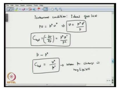
Now, if the change in the pressure is negligible that means let us say P is not very different than  $P^*$ , we can say the hydraulic capacitance will be  $V^*$  over  $P^*$  and this is when pressure change is negligible, right. So at time t=0, the pressure is  $P^*$  everywhere as we told in the beginning and as pressure of liquid increases, so the pressure will change from  $P^*$  to  $P^*$  delta P, right.
