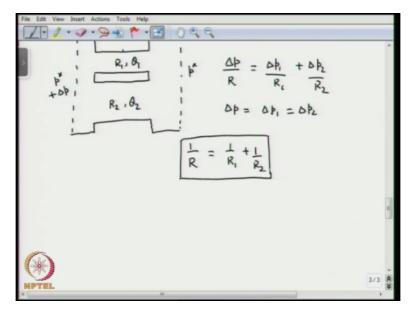
So when they are connected in parallel, let us consider this case here, okay. So, this is P\* + delta P, this is P\*, so that these are 2 channels, this is channel 1, this is channel 2 they are connected in parallel, this is R1 and R1 is the resistance and Q1 is the flow rate, here is R2 and Q2. So, you can write Q the total flow rate is going to be Q1+Q2, right. So, you can write delta P over R is going to be delta P1 over R1 + delta P2 over R2.
