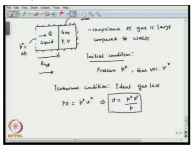
So, we would consider this situation here, okay. This is a rigid wall, so we are not you know talking about deformable walls, we are all interested in how the pressure is varying for the gas. So this is the gas, let us add some instant, the pressure P and the volume is v, this is the liquid, which is moving at flow rate Q and this is that liquid. Here, the pressure is P\* + delta P and till here we say the hydraulic resistance is R hydraulic.
