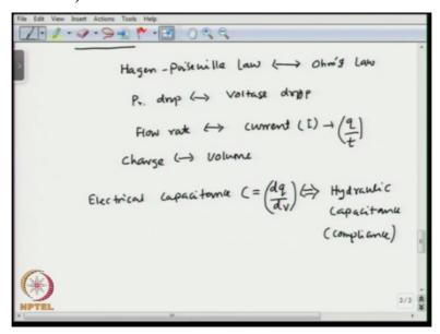
The change in the voltage, which is equivalent to the term called hydraulic capacitance or it is also known as compliance, okay. So, compliance can be defined as, compliance is denoted by c hydraulic is - dv over dp, okay. So, here we notice that there is a negative sign here and the negative sign is because as the pressure increases, the volume diminishes, okay. So, the volume and pressure inversely proportional to each other, so there is a negative sign there.
