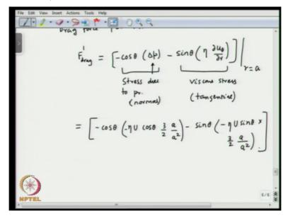
I am writing is as delta P, okay = - eta \* u \* 3/2 a over r square \* cosine theta. So this is the pressure field. So now, if you want to find out drag force per unit area, you can find F drag per unit area use the dash symbol = -cosine theta, so that makes it normal to the surface \* delta P, right - sine theta \* eta delta U theta over delta r. So, essentially this is the stress that is coming because the fluid pressure.
