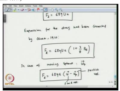
So if you look at this velocity component as r increases, so the velocities ideally should become free stream velocity, so that is not happening so that needs some corrections. So the expression for the drag has been corrected by Oseen in 1910, where he said that the drag is
