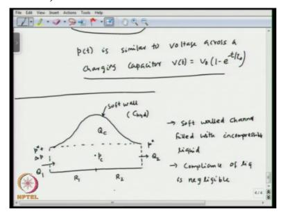
Now, let us look at another example where we talk about a chamber with a flexible membrane, okay and we would see how the pressure of the chamber is going to vary with time, okay. So, we consider another example of a chamber with a flexible membrane, let us say this is the flexible membrane, okay and this is the inlet, this is the outlet of the channel. Now, let us say the pressure here is P\* + delta P and the flow rate is Q1.
