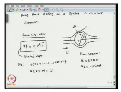
You would like know what is the quantitative expression for the drag force that is acting on microparticles, okay. So let us consider this example, so we have a sphere which is present in an infinite domain, so say this is some r, this is theta, this is radius a, so you would have flow situation something like this. So the pressure force always acts normal to the surface and there will be a viscous component tangency here, right.
