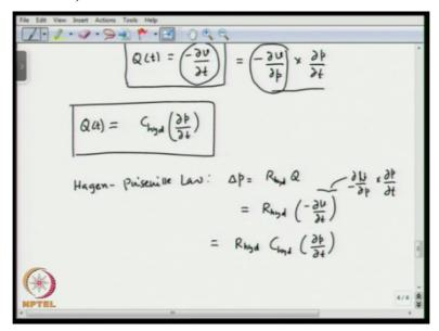
Now, so this is what we found, if you use Hagen-Poiseuille law, you can relate delta P to be R hydraulic \* Q, right. So you can write delta P = R hydraulic \* Q, which will be = R hydraulic \* Q, you can write it as - delta V over delta t and so this you can also write it as = R hydraulic \* c hydraulic \* delta P over delta t, right. You can write it as delta P over delta t, right.
