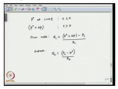
And when the inlet pressure changes to  $P^* + \text{delta } P$  then the membrane is on deforming. So the flow rate Q1 that is coming in at the inlet =  $P^* + \text{delta } P$  - Pc is the central pressure divided by R1, right and similarly, at the outlet, you can write Q2 will be = Pc -  $P^*$  divided by R2, okay. So from here, you can find the rate of volume expansion which is same as the dead volume created here because of the expansion of the membrane, right.
