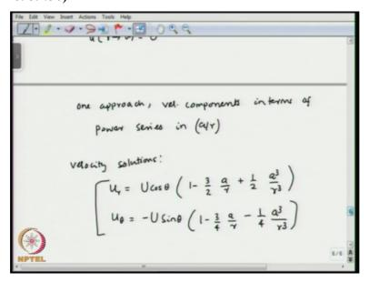
One approach would be to expand the velocity in terms of the ratio between the radius of the circle divided by the radial coordinate, okay. So, one approach so velocity components in terms of power series in a over r. So we can write down the velocity solutions in power series
