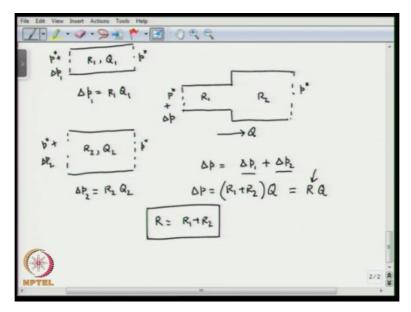
So, we consider hydraulic resisters in series and parallel, okay. So, let us consider 2 channels first, 2 individual channels, so this is let us say channel 1 and here, the pressure drop is  $P^* + \text{delta P}$  and the pressure  $P^*$ , so the resistance is R1 and flow is Q1, so you can write delta P, let us call it delta P1 = R1\*Q1, right. So now, we consider another channel which is little bit wider and here, we have  $P^* + \text{delta P2}$  and here the pressure is  $P^*$ .
