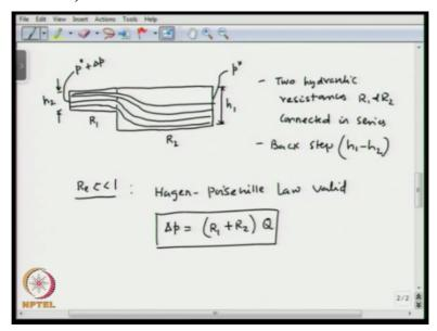
And this segment is R2, okay. So here, the pressure is P\* + delta P and here the pressure is P\*. So, we have 2 hydraulic resistances R1 and R2 connected in series, right. So and that form say back step, okay. So the back step height is h1-h2, okay. So, we consider the first case, okay where the Reynolds number is << 1, okay. So in that case, the Hagen-Poiseuille law valid.
