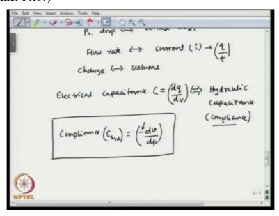
Now, compliance has you know importance in design of microfluidic system, you know if you are not talking about ideal fluids, all real fluids have some degree of you know compliance, so that can be compressed to some degree. Also, if you are talking about in a microfluidic channel with flexible walls, the walls that are not very rigid or we talk about in a
