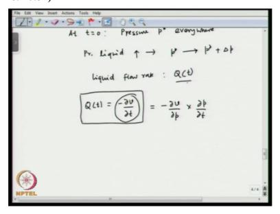
So, the liquid flow rate, as pressure will change, the liquid flow rate would be Qt, right. So, Q will be a function of time and this fluid flow rate would be nothing but the decrease in the gas volume, so as we see here as the liquid is advancing, the gas volume is going to reduce, so the
