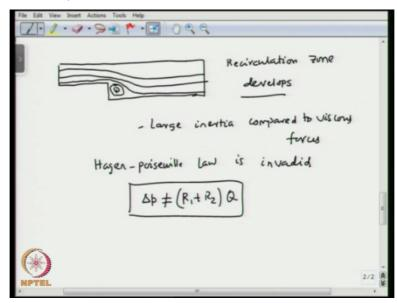
So, L be a recirculation zone forming there and in that case, so here we would have recirculation zone develops and this is because when Reynolds number is >> 1, we have large inertia compared to viscous forces, right. So in that case, we cannot apply Hagen-Poiseuille law. So, Hagen-Poiseuille law is invalid, right. So in that case, we cannot write delta P = R1+R2\*Q, okay.
