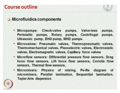
In the following chapter, we will talk about microfluidic components, different microfluidic components like micropumps, microvalves, microflow sensors and micromixers. Micropumps are components that is used to drive fluid through microfluidic devices, microvalves are used to manipulate flow in micro devices, microflow sensors are used to measure flow rate in microfluidic devices and micromixers are used to mix fluids in micro devices.
