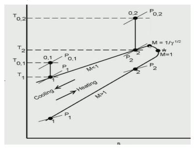
So, to summarize what we said earlier state point 1 if it is supersonic it lies here the Rayleigh line is steeper than the Isobar which passes through this and the slope approaches +infinity as we approach M=1. Subsonic state lies above like this and the Rayleigh line is less steep than the Isobar here is the Isobar corresponding to P=P1 the Rayleigh line is less steep than that and the slope keeps increasing.
