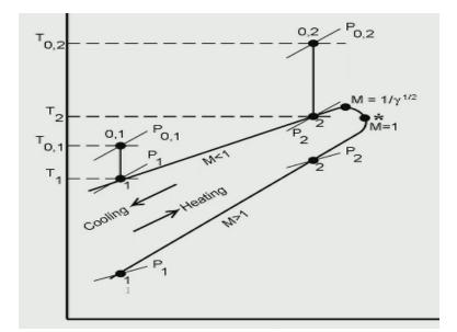
So, we are starting with we are starting with state 1 remember this is a supersonic state which is why it is down here and notice that the the Isobar is less steep than the than the Rayleigh line, So, the Rayleigh line is shown here using a thick black line as you can see from here and the Isobar which is this one here is less steep than the Rayleigh line and this is the supersonic branch.
