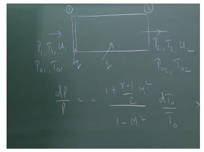
Where we were looking at flow situation like this? So let us say this as duct or a pipe in which heat is added and at entry the flow is at state 1 and at outlet or exit flows is at state 2 and starting from the inlet state which was at p1. Let us say T1 u1 and P01 T01 we wanted to find out the exit state which is P2 T2 u2 and P02 T02. We would like to do this for 2 conditions one when the inlet flow is sub sonic
