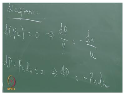
So, we will start with the differential form of the governing equation in order to do this. So, we will illustrate. So, if you remember the differential form of the continuity equation was d of rho u=0 right from which I can write d rho/rho=-du/u. Okay the differential form of the momentum equation looks like this and if I rewrite this I can write like this.
