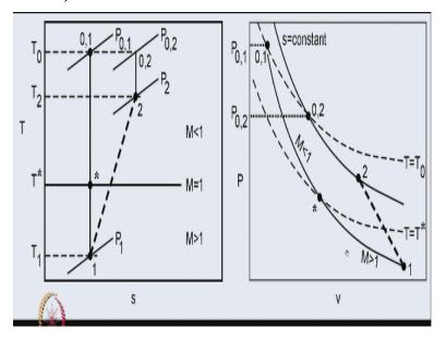
And these are the 2 diagrams that we are looking at the state 1 here is the state ahead of the normal shock and state 2 is the state behind the normal shock this is illustrated on a TS diagram here and we illustrated in the same thing on a PV diagram again. state 1 denotes the state ahead of the shock wave and state 2 denotes the state behind the shockwave. One important aspect about this diagram is that although we have connected states 1 and 2 using a line.
