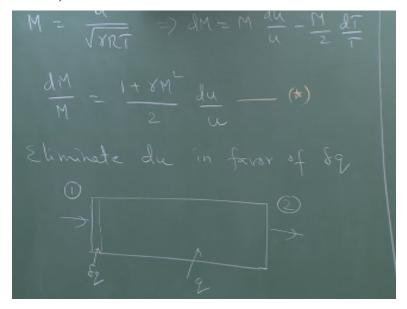
And that we can get from the definition of Mach numbers M=u/square root gamma RT and if I take the derivative of this right I can write dM=M times du/u-M/2 times dT/T. Now once again substitute for du/u and dT/T from before this gives me dM/M=1+gamma M square/2 times du/u. So, the nice thing is what we have done is for an incremental change in du I know how to calculate the changes.
