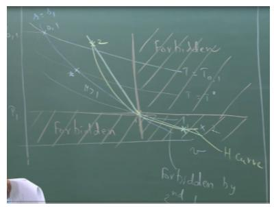
So, this is the H curve. So, notice that this was state 1 so. of intersection of the straight line with this H curve state 1 of intersection of the H curve with straight line and H curve gives me state 2. So, this is state 1 this is state 2 okay what is that there is also a point of intersection on the side of this is another Rayleigh line. You will get another state point 2 here but as we said earlier this solution is not allowed by the second law of thermodynamics.
