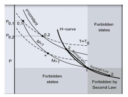
So, this is what the solution looks like, so you can see the features that we already discussed. So, this is state point 1 right and you see the Rayleigh line which is the straight line here on this side and the Rayleigh line which is the straight line on this side and states downstream states 2 are not state 2 is not allowed to lie in this quadrant or in this quadrant. As we discussed earlier, and it can actually lie in this quadrant where such a solution would employ  $s_2 < s_1$ .
