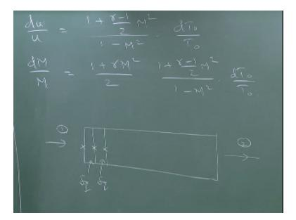
And then du/u=1+and dM/M. Now, the equations are in the form in which they want them I can calculate for a given an addition of heat delta q. I can calculate change in density, I can calculate change in pressure, change in temperature, entropy, velocity, and Mach number. Okay so this is exactly in the form in which I want these equations. So, what we are going to do next is for addition or heat removal in the flow.
