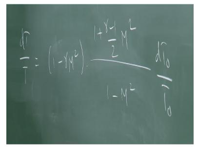
I get d rho/. rho= so when the stagnation temperature changes by this amount dT0 which is the result of an addition of heat which is delta q the density changes by this much. Okay similarly dp/p=-gamma M square times 1+gamma-1/2 times M square /1-M square times dT0 over T0. So, this is how much the pressure changes as a result of an addition of heat which is delta q right. And now I can look at change in static temperature dT/T=1-gamma M square times 1+gamma-1/2 times.
