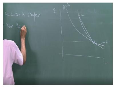
So, let us say that this is state point1 and let us say this is the isentrope which passes through state point 1. Now, remember the H curve is actually steeper than so this is state point 2 and this is the H curve since the H curve is steeper than the isentrope. Since it is steeper for a given change in specific volume v1-v2 the change in pressure this is p1 and this is p2 had we compressed using a isentropic process we would have remained on this is s=s1.
