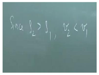
Rho 2 is > Rho 2, that we have already shown, so since rho2 is > rho1, v2 is going to be; the specific volume is going to be < v1, so that means that state 2 is going to lie above and to the left of state 1 but it is going to lie on a different isentrope because the entropy increases across the shock wave. So, we draw a different isentrope, which looks like this.
