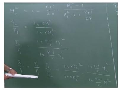
And if you remember, the solution looks like this, we wrote down M2 square downstream of the shock wave as 1-gamma +1/ 2 gamma times M1 square-1 divided by M1 square-1+gamma+1/ 2 gamma. This was the solution for M2 for a given value of M1 and the other quantities, we wrote down earlier, so let me just rewrite them here; P2/P1 = 1+gamma times M1 square divided by 1+gamma times M2 square.
