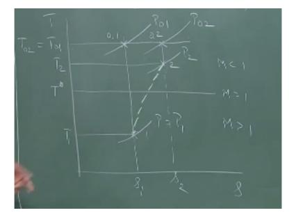
In addition, we know that downstream on the shock wave, the flow is subsonic. So, when we illustrate these state points on the TS diagram, all these information must be put in. So, let us see how we go about doing that. So, first we do this on a TS diagram, let us say that for the given state P1 and T1, say that this is T1, this is the isobar corresponding to P1, so that is the initial state 1 and let us say that this is s1.
