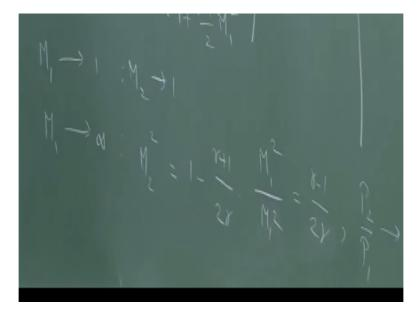
So, I substitute that value into this expression and if I simplify, I get the fact that rho2/rho 1 tends to be gamma+1/gamma – 1, okay. So, I substitute for this M2 square from here and if I put this in, I am sorry; they do this correctly, oh! I am sorry; yes, please make a small correction, this one should be gamma -1/2 gamma this is also M1 square but this is gamma -1/2 gamma.
