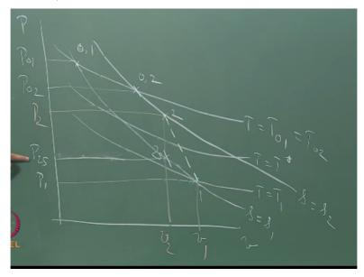
Now, let us look at this diagram a little bit in slightly more detail to get an idea about the effectiveness and the efficiency of the shock wave compression process okay. Now, if I look at state 1 and 2, notice that the change in specific volume, so this is v2, this is v1, so from a given state, this is the change in specific volume and you can also see that this is P2. So, the normal shock compresses the gas from P1 to P2 with this much change in specific volume, correct.
