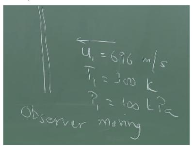
The observer is moving, so we go to that kind of a frame of reference, which looks like this, so here observer; so this is still 1 and this is still 2, so in this case; so this velocity u1 is going to be 696 meter per second, right. So, the wave has become stationary, so the observer perceives the flow to approach with the speed of 696 meter per second, correct. So, initially the wave was moving like this at 696 meter per second.
