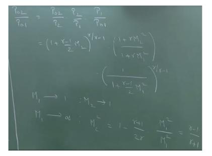
One additional quantity which is of importance in normal shock calculation is the ratio of stagnation pressures, downstream of; or upstream of the shock wave and if you recall, this can be written as P02/P2 times P2/P1 times P1/P01 and P02/P2 can be written as 1+gamma - 1/2 times M2 square raised to the power gamma over gamma -1 and P2/P1, we can write from here, so that is =, 1+gamma M2 square divided by 1+gamma M1 square and P1/P01 can be written in the same way.
