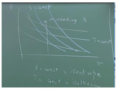
And what we are going to start with today is to depict say, same states on a PV diagram; on a PV diagram then we would like to show just like this, we would like to show; s = constant, which is an isentrope line on this diagram and also an isotherm which is at T = constant on this diagram. So, that is what we start out with and if you remember the equations that we wrote down for change in entropy, let us start with that equation.
