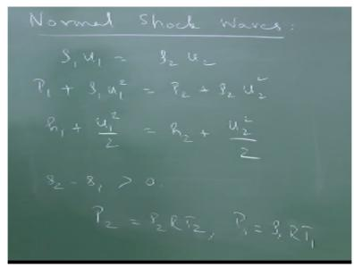
In other words, what are the velocity of the fluid, pressure, temperature and so on at state 2 given the information in state 1, that is what we are looking for and we use the same governing equation as before, if you remember the continuity equation looks like this and the momentum equation, the energy equation and if you remember the change in entropy, we are saying that the change in entropy must be positive.
