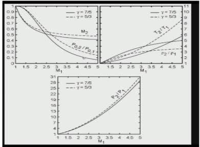
So, we can actually look at this figure and see how the various quantities depend upon the gamma, so here we have illustrated quantities like Mach number downstream of the shock wave M2, stagnation pressure downstream of the shock wave here, ratio of temperatures across the shock wave ratio of densities and P2/P1 for the different cases, you notice that for P2/P1, there is another significant difference as Mach number increases in these cases, right.
