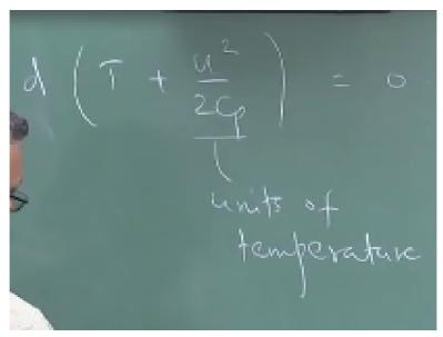
I can write this as, T + u square / 2cp = 0, in the absence of any heat addition, right, I can write this, so the quantity u square/ 2cp has units of temperature, same as T, right. So, this has; this quantity has units of; so this gives me an idea as to how I can illustrate velocity on a TS or a PV diagram, so I simply calculate u square/ 2cp and I add that to the static temperature, right.
