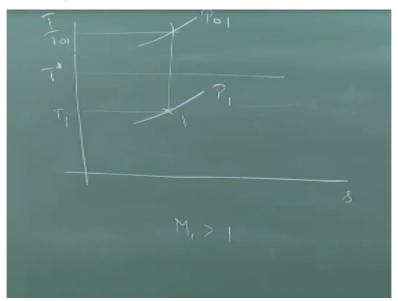
So, it is an extremely powerful way of illustrating the process and states for the type of flows that we are going to encounter. Now, had the initial state being a supersonic state, right, how would this have looked? I would have gone through the same process but my diagram would be slightly different, if M1; so this is my TS diagram, if my initial state had been a supersonic state and I would have depicted state 1 like this, so this is T1 and this is P1, so this is T01 and this is P01.
