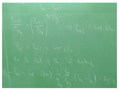
Eta turbine = T04 - T05 divided by T04 - T05s. So I can calculate T05s from this expression. I know eta turbine also. Eta turbine is given to be 0.9 so I can calculate T05s from this can you calculate this and let me what it comes out to be? To5s is 1017 Kelvin. That is T05s. So once I know T05s I can calculate P05s using the isentropic relationship. So if you remember T05s divided by T05 = raise to the power gamma g - 1/gamma g.
