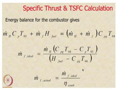
So the fuel consumption for the engine can be obtained by doing an energy balance for the combustor. So, if you will get the combustor at steady state operation so you have mH dot, amount of air coming in at a stagnation temperature T03 and we have a certain amount of fuel mf dot which comes in with negligible velocity, but with calorific value given by this amount. So this is the rate at which energy is being brought into the combustor by the fuel.
