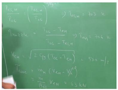
So I can write Pes for the hot nozzle divided by P06 = Tes for the hot nozzle divided by T06 to the power gamma g/gamma - 1. From this I can calculate my Tes for the hot nozzle. So what you get if you do this calculation. gamma g/gamma g -1 and what do you get for Tes, H this is correct is it 703. So, the efficiency of the nozzle if you remember is T06 - Tes divided by T06 – Tes, H so from this I can calculate my Tes.
