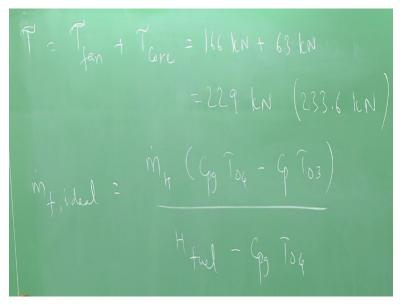
So total thrust T = Thrust produced by the fan + thrust produced by the core engine and this comes out to be 166 kilo Newton+63 kilo Newton which is = 229 kilo Newton which encouragingly compares extremely well with the value reported by the manufacture. So the manufacture quotes static thrust value for this engine to be 233.6 kilo Newton.
