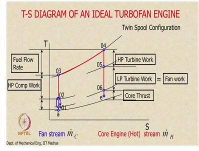
So if it is 30, 40 augmentations that means the actual value is as we are seeing here 150% of this right, is we will follow this up with a look at the TS diagram of an ideal turbofan engine okay. And the turbofan engine as I said earlier has multiple spools because of the differential speed requirements of the fan and the compressor blades, so the fan has to spin at much lower RPM whereas they are the last stages of the compressors have to run that much higher RPM.
