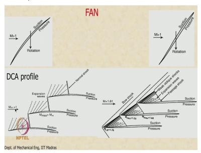
So in the last class, we saw that double circular arc profile cannot be used for diffusing a supersonic flow, and we showed that because it has the contact surface here by the time the flow reaches the entrance of the blade passage which is over here, you can see that the maximum Mach number is going to be more than the free stream Mach number probably much more than the free stream Mach number.
