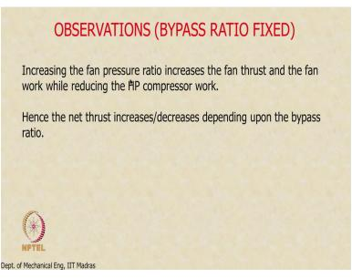
The next effect is keeping bypass ratio fixed what happens if I increase the pressure right, now that also we can see from here, now increasing the fan pressure ratio increases the fan thrust and
