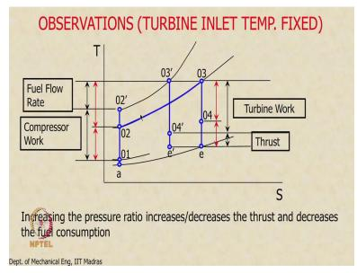
So we will keep the turbine inlet temperature fixed, this is the basic cycle that we saw earlier, so what we are going to do now is we are going to keep T03 same, we will keep T03 the same and we will increase the pressure ratio okay. So let us see what happens, this is compressor work now the compressor work will also change because we are increasing the pressure ratio right, so this is the earlier value for the compressor work and turbine work.
