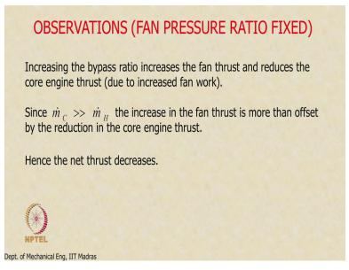
Now if you think about this in the earlier turbojet cycle we identified 2 parameters in the cycle, one was the pressure ratio, other one was the turbine entry temperature. Now with a turbofan cycle and we looked at the effect of increasing the turbine entry temperature on the performance of the cycle, and the performance was assessed based on fuel flow rate and specific thrust or thrust itself that was so we looked at the effect of increasing turbine entry temperature on these 2 matrix.
