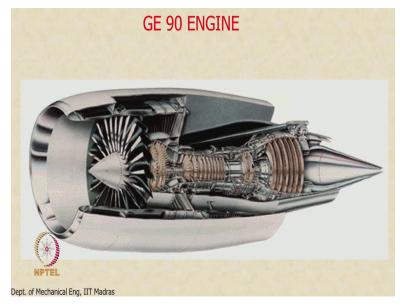
The next engine that we will talk about is the GE90 engine, which is probably the biggest engine that GE offers next only to the Gen X engine which is the latest offering. This is probably the largest engine in service today the biggest engine in terms of thrust produced, biggest engine in service. You again see the same kind of thing the fan, the moving blades of the fan, the stator blades of the fan and the fan nozzle.
