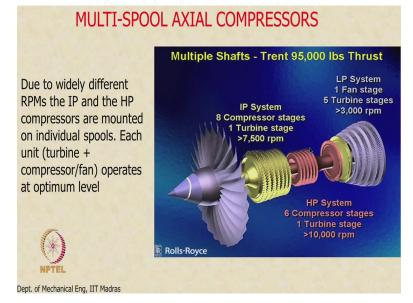
So because we have widely different requirements for RPM right, the only way we can actually meet this challenge we want the fan to run at low speed at the same time the other components have to run at a higher RPM, so only way we can accommodate such widely differing RPM used to have the Multi-Spool technology. So there were the first technological challenges that had to be overcome, and it was overcome by using a revolutionary technology called the multi-spool technology.
