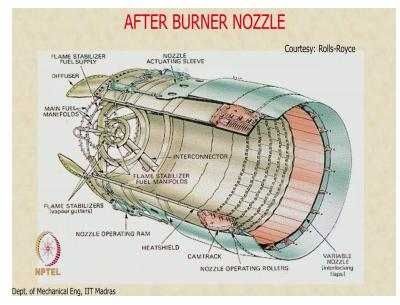
Today, we will start our lecture by looking at the nozzle for and after burner, the nozzle for the after burner has to be little bit more special because it has to accomplish in addition to the 2 things that we talked about, for example we said that the purpose of a nozzle is to produce thrust and also it must be used for thrust reversing. Now an after burner nozzle will not have the capability to have thrust reversing, so it will produce thrust.
