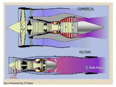
So here is a pictorial view of a high bypass ratio engine and low bypass ratio engine, the low bypass ratio engines are typically employed for military applications, and the high bypass ratio engines are typically employed for commercial aviation applications okay. You can see the increase in diameter with increasing bypass ratio, and the consequent increase in the frontal drag okay.
