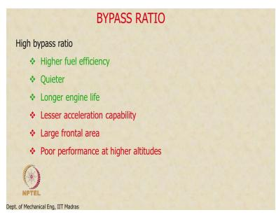
So not all actually is good for the bypass engines okay, so if you look at the high bypass ratio turbofan engines definitely higher fuel efficiency because the propulsive efficiency is better. And the engines are also quieter because as I said the cold air mixes with the high speed hot air thereby reducing the velocity gradient, when the stream comes out of the engine and mixes with the ambient, so the aerodynamic noises has brought down.
