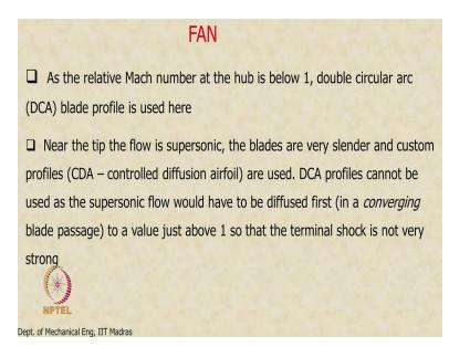
So the relative Mach number at the hub is below 1, so normally the blade section okay the blade section is made up of 2 circular arcs okay, so this is called as double circular arc profile for the subsonic section it is called DCA blade profile.
