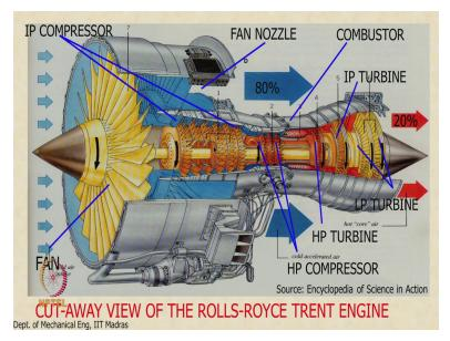
A comparable size engine here is an offering from Rolls-Royce, the similar rating you see the big fan in different. Rolls-Royce typically tends to use 3 shafts okay we will see why in a minute, so this is the fan, then there is an intermediate pressure compressor as you can see, and then there is a high pressure compressor, high pressure turbine, intermediate pressure turbine and low pressure turbine.
