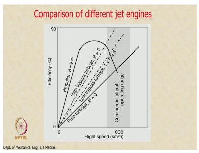
Let us take a look at some more concepts and then see why bypass ratio engine or bypass turbofan engine makes sense okay. So here I have plotted propulsive efficiency versus flight speed, remember we said that we wanted the flight speeds to be in the high subsonic Mach number range, so that means we are typically talking about flight Mach number of about 1000 km per hour or so, and altitude of about 35000 feet, 35 to 40000 feet no more than that okay.
