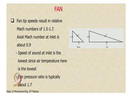
And we have supported the difference in speeds with multiple spool technology okay, but the challenge is do not stop there, let us say that this spin the fan spins at 3000 RPM, now unfortunately because of the bypass ratio that are required remember the diameter is determined by the bypass ratio, now we know the speed so which means I can determine the tip speed as you know that fan tip diameter is about 2 meters or so knowing the RPM I can determine the tip speed.
