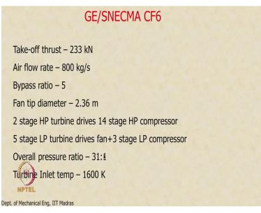
So some of the specs of this engine we can see that it is a low bypass ratio engine bypass ratio of 5, handles about 800 kg per second at take-off, fan tip diameter as you can see how big it is? It is about 2.36 meters, so you can imagine the fan blades are quite big right. So we have 2 stage HP turbine which drives 14 stage HP compressor, 5 stage low pressure turbine drives fan +3 stage low pressure compressor.
