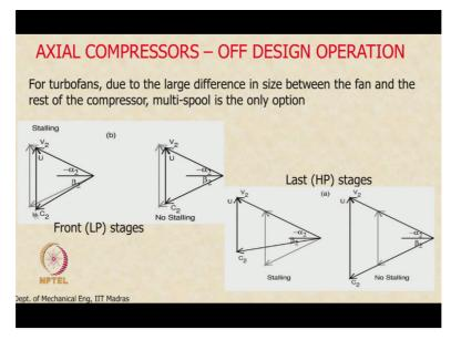
That is another strategy, which is also utilized in the industry so we can see here this stalls right because we have kept the blade speed the same, the angle the same, this one stalls. The velocity vector swings this way. What if I reduce the blade speed? Keep this angle the same, stator blades are fixed, I change the blade speed slightly now the velocity vector will line up nicely and in this case it stalls because I have kept U fixed and also alpha 2 fixed.
