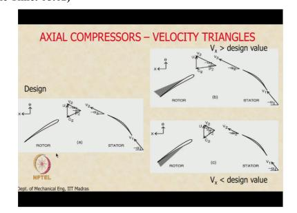
So on the left here you see the design velocity triangle, so you see this stator blade, this is called as stage, a stator+rotor combination is called a stage. So you see the stator so all the stator does is deflect the velocity. So the fluid comes in with an absolute velocity V1 and with the angle of inclination alpha 1 like this and the stator deflects the flow keeping the magnitude the same.
