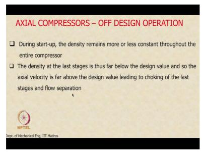
So when the later stage is choked then we have problem. As you know, once the latter stage is choked, we cannot push anymore mass flow rate into the system because they are already choked right. We cannot have any more mass flow rate pushed into it, so we run into a problem. So here what is happening is the actual axial component of velocity remember mass flow rate is m dot s rho times A times Vx where Vx is the axial velocity.
