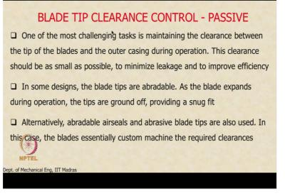
So how do we maintain the blade tip clearance control? Two strategies are possible, 1 is a passive strategy okay and as I said this is probably one of the most challenging tasks in the manufacturer and operation of a compressor okay. So the clearance should be as small as possible as we said to minimize leakage. So the air leaks around the top of the blade, it is not going to increase its pressure, it is of no use to us right.
