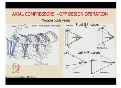
So that is what we mean by variable stator blades okay or movable guide vanes as it is called okay. It is also called movable guide vanes. So here let us look at this and then we see how it is actually implemented in an engine. So here as we can see we are looking at this type of a situation right. So you see that this is the design velocity triangle, the 1 in grey is the design velocity triangle okay.
