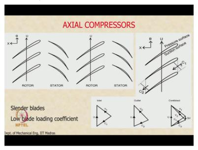
And we saw that under design conditions, the pressure rise across the compressor stage. Each stage is about 1.15 and we also saw that the compression process is primarily due to diffusion of the relative velocity. So the relative velocity magnitude decreases from C1 to C2, there is a reduction and there is also increase in the cross-sectional area, which causes the pressure to increase.
