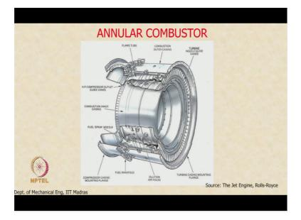
Now the next one is the annular combustor okay. So here you can see this side connects to the compressor, this side connects to the turbine and you see the passage for the shaft, you see the inner casing, you see the outer casing, and then you see the liner. So here is the liner, liner on the flame tube. So this goes in the entire circumference. Combustion takes place across this annular space right.
