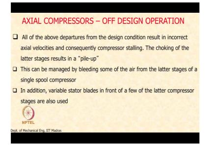
That is what we are going to look at next. So to sum up what we just said so all these above departures whether it is above the design point or below the design point causes incorrect axial velocity and compressor stalling. We saw that the blades are stalling. Choking of the latter stages results in pile-up meaning it is already choked so it cannot really pass more mass so it causes the flow to build up in the later stages of the compressor.
