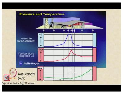
That is a widely used industry practice and if you remember we saw this earlier when we looked at the slide we can see that, so here are the compressor blades. The fan, the intermediate pressure compressor and the high pressure compressor and you see that the axial velocity here more or less remains constant definitely up to entry into the combustor. So it is always good to design these for constant axial velocity.
