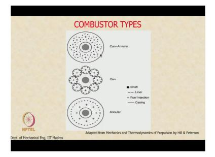
Now in aircraft engine, 3 types of combustor designs are possible okay. The common elements in all the 3 design is that you have for example here we are looking at the combustor (()) (36:44) so this is the shaft right. The one in the center the grey circle is the shaft, so I am looking at the combustor from this end or the other end, so this is an end view of the combustor.
