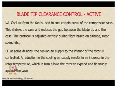
So you control the expansion and shrinking of the disk and the blade in a controlled manner by sending air into the compressor case or into the rotor, both are possible. You can send air into the compressor case, which is on the top or you can also send air into the rotor, which is also hollow. So by controlling the amount of air so this is done actively during flight based on many of the settings that you have, altitude, rotor speed, flight speed you know engine condition and so on.
