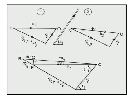
And at this solution also which is the expansive solution. So, here the velocity vector after passing through the wave is deflected away from the wave so this is an expansion solution and based on these 2 triangles we derived some relationship. Let us just recap these things quickly. (Refer Slide Time: 00:51)
