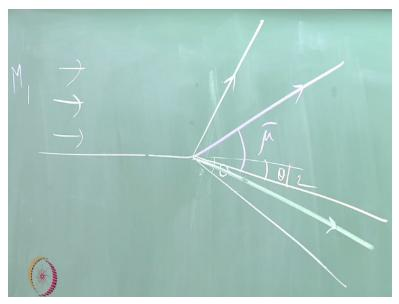
So these were the initial and final Mach waves and let us say that this is my, this angle let us say is theta/2. So the single wave that replaces all this looks like this and this angle is mu bar. So that angle is measured with respect to theta/2 so that is mu bar. So we replace this entire fan with the single wave like this. This is an approximation such a solution is not allowed, but it is an approximation.
