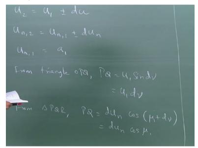
We wrote u2 to be u1+or -du and we also wrote un,2 as u n1+or-dun and if you remember un,1 in both cases is = a1 which is the speed of sound of the flow approaching the wave and based on the triangles for example based on triangle OPQ so from triangle OPQ we wrote PQ = u1 sine d nu and for small values of d nu this can actually be written as u1\*d nu and from triangle PQR.
