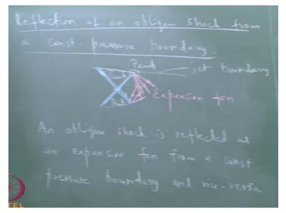
Before we do that we need to look at one concept which is reflection of an oblique shock from a constant pressure boundary. In the previous chapter, we had looked at reflection of an oblique shock from a wall or a solid boundary and we saw that an oblique shock is reflected back as an
