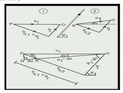
So this velocity triangle that we have here corresponds to the this is the combined velocity triangle for a compressive wave solution because as you can see the flow after passing through the wave is deflected towards the wave. So, this is the compressive solution.
