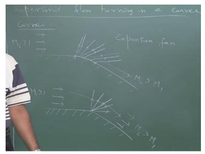
Next we are going to look at supersonic flow turning in a convex corner. "Professor - student conversation starts" Sir, flow passing through an oblique shock will have a higher pressure downstream of shock and flow passing through isentropic compression will have less pressure, but about the slip line the pressure should be same. No, here in this case, you cannot say that the pressure after the oblique shock is higher.
