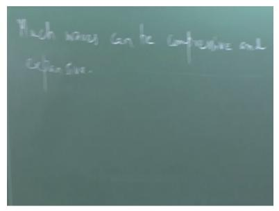
So Mach waves can be compressive and expansive. In the earlier situation that we drew when we looked at a point disturbance which was traveling with supersonic speed that was traveling with a constant supersonic speed, but if it starts accelerating then we are going to degenerate different Mach cones. So if it starts accelerating then the Mach waves that it would generate would look like this.
