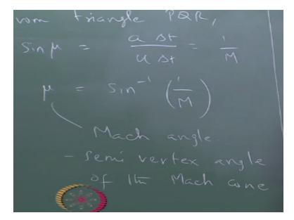
So from the triangle PQR in this figure, we can see that sine mu = a delta t divided by u delta t that is 1/m so that mu is arc sin 1/the Mach number and this mu is called the Mach angle. Note that mu is not the flow deflection in this case. The flow is deflected through a very small value, much smaller than mu. So mu is the semi vertex angle of the Mach cone. So this is the. The other point that I want you to note from this diagram is that the point R.
