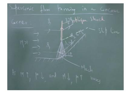
The waves are actually going to intersect and normally the way this happens is so here is our first wave, here is our next wave so this is how the waves normally do. So they actually intersect at a point. I am not going to show this, but that is what happens. So these are Mach waves. I have shown only a finite number, but what you must remember is the reason for discussing the earlier theory.
