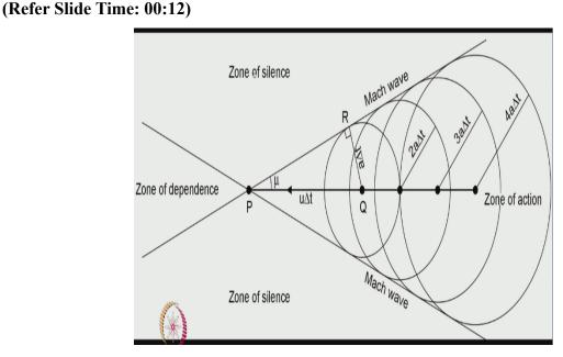
In the last class, we looked at the Mach cone and the propagation of disturbances from an object which was moving with speed greater than speed of sound. So this is the point disturbance which moves with the speed which is greater than the speed of sound and these are the spherical wave fronts of sound waves which were generated at an earlier incident and time, and as you can see from this triangle PQR you see that the radius of this triangle.
