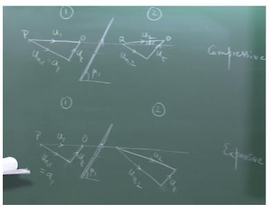
So let me call this is this is the direction, let me call this region 1 and region 2. Let us call this u1, this is normal to the wave and what did we say earlier about the normal component, the normal component is equal to the speed of sound. So this is the normal component and this is = a1. This is the tangential component ut and this angle is the wave angle mu1 correct. So as I said the
