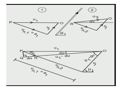
Here it is so you can see the same construction 1 and 2. This is the velocity vector before un1 = a1 ut. This wave angle is the Mach angle mu1 and after passing through un2 decreases is < un1 so the velocity vector shifts that way because ut is the same. This angle is dnu and I have combined these 2 triangles by merging these 2 sides like this and you see the same construction so u2 is u1 - du.
