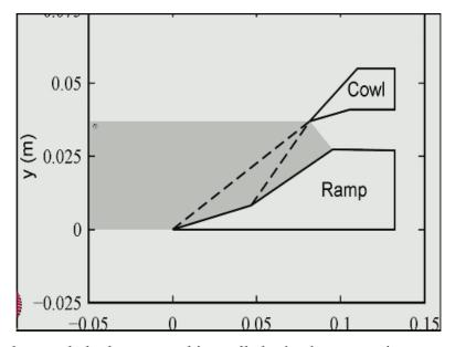
The next worked example looks at something called mixed compression supersonic intake for may be ramp jet engine. So you notice that these are 2 things here one is called the Ramp and the other one is called the Cowl. So the freestream approaches the intake this way and notice that when the freestream comes here that is one deflection of the supersonic flow here so the freestream is at the supersonic mach number.
