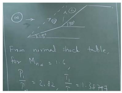
So let us make a sketch of the flow situation. So we have this is the first shock this is the second shock. So we are labeling this region as infinity. So this is how the velocity vector looks like ahead of this shock wave the direction in this shock wave is like this, the direction in this shock wave is like this. So we call this region 1 and we call this region 2. So this is the cowl which starts from there.
