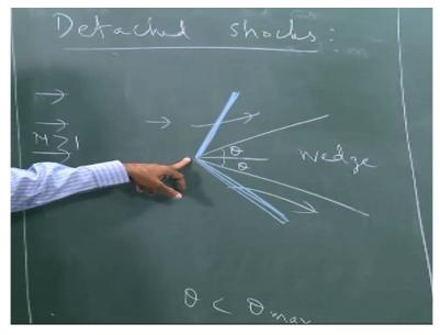
So we move on to the next topic which is Detached Shocks. So all the solutions that we have looked at so far are attached shock solution. In reality as we said earlier when theta flow deflection angle is greater than theta max for that particular mach number the shock becomes detached. So obtaining a solution for this case is very complex and because the flow is much more complicated than what we are assuming.
