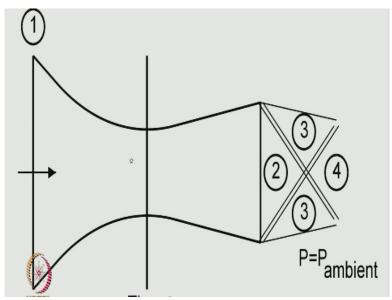
And that worked example is shown here in this figure. We had a convergent, divergent nozzle with the exit to throat area ratio being given and starting from state 1 we evaluated the mach number in the pressure and for the ambient pressure which was given be 100 kappa. We notice that for that ambient pressure the jet was over expanded. So oblique shocks are triggered.
