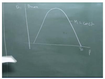
If I draw the theta beta M curve corresponding to this mach number remember this is for an attached shock solution this is a detached shock wave. So the inferences for that reason are going to be only qualitative what this suggest to me. There are two things that we have said and we can actually infer from here to here based on the two things that we have discussed so far. We will pick it up in the next class and then continue from there.
