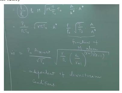
If I expand this equation further I can write this as I am sorry rho/rho 0 times rho 0 times M times square root of gamma R T/T0 times T0 all within the square root times A/A star times A star. Notice that rho/rho 0 is known to us as a function of Mach number right, we know the relationship T/T0 is also known to us as a function of Mach number, A/A star is also known to us as a function of Mach number, area Mach number relationship.
