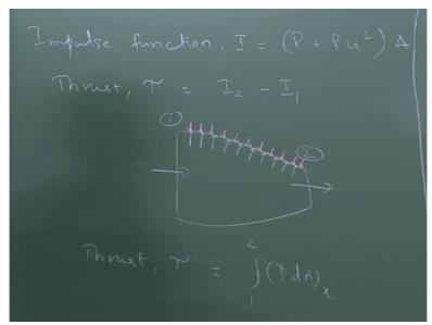
In the last class, we showed that the impulse function I, which was defined as P + rho u square\*the cross sectional area on the stream tube at that location, can be used to calculate the thrust that is produced, thrust or drag that we get from different components, and the thrust could be evaluated as I2 - I1, where the state point 2 refers to the exit of the device, and state point 1 refers to the inlet of the device.
