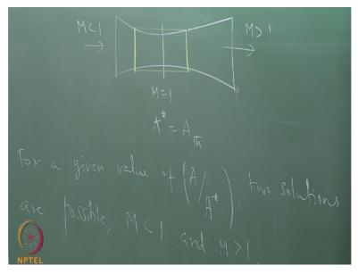
That is also clear if you look at the same flow situation. So for example, if you look at a flow situation like this, where M=1 and if for example the flow enters at a subsonic Mach number and exits with a supersonic Mach number, then the A\* in this case = A throat. However, if I consider 2 sections like this, this cross section and this cross section, notice that A/A\* for both these cross sections are the same.
