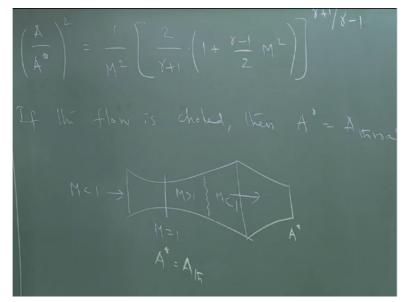
This is the so called area-Mach number relationship where we have the area term on the left hand side and the Mach number term on the right hand side. Here  $A^*$  is the area or cross section where the Mach number reaches 1 and as I said earlier,  $A^*$  need not be = A throat. If the flow is choked, then  $A^*$  is indeed = A throat, otherwise we have to determine  $A^*$  in some other manner.
