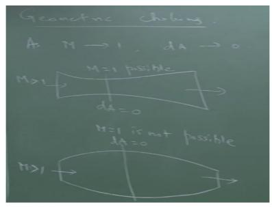
We have looked at thermal chocking where enough heat addition could cause the Mach number could go to 1 either from a subsonic Mach number or a supersonic Mach number with enough heat addition we can make the Mach number go to 1 or the flow attains a sonic state. We saw with friction also that if you make the pipe long enough we can attain the sonic state in the pipe if you make it long enough, now that was friction chocking.
