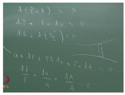
The next topic that we are going to take out is area velocity relationship, which is a very important relation when dealing with flow through varying area passages. So here we try to determine the relationship between changes in velocity and changes in cross sectional area. So what happens when the cross sectional area decreases, or what happens when the cross sectional area increases, that is what we are going to try to figure out.
