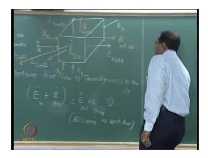
So, applying the 1st law thermodynamics, should the CV, the control volume, and putting E dot because this heat transfer we are talking about, rate per second, the transfer, that is what we are interested, what is joule per second. So, E dot in, what is, whatever the energy is coming in plus, these are correct.
