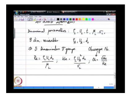
I have liquid density, liquid velocity, liquid prefilmer thickness, liquid viscosity surface tension potentially, but in addition I also have the air side properties, the air density, air velocity, the airside length scale like a diameter of that inner air passage actually I could even include air viscosity.
