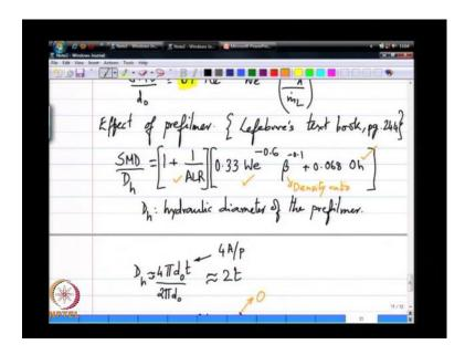
So, if I take the prefilmer, this is the area of the prefilmer, the hydraulic diameter is approximately equal to 2 times t.
