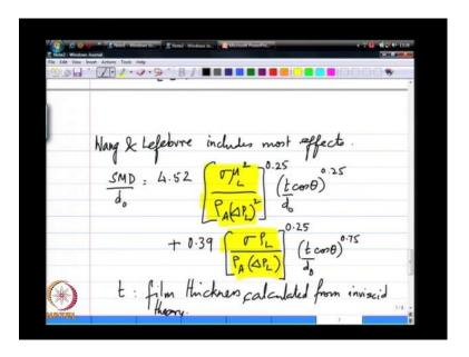
And the one due to Wang and Lefebvre is the most general in this regard, and what that gives us t here is a film thickness, that can be obtained from inviscid theory. Now these quantities that you see in this parenthesis, actually I need to face that, so that case be the dimensionless film thickness, these quantities inside the square parenthesis, this part and this part are essentially dimensionless groups that are functions of the Reynolds number and Weber number.
