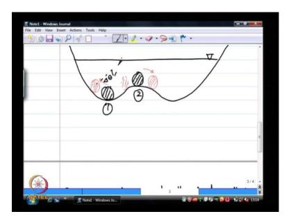
I will redraw the figure here just for clarity, if I displace it slightly, what the ball will do is essentially trace it is way back towards equilibrium condition 1. If I apply the same logic to this, if this is the direction of displacement, the ball is going to or the ball is going to move away towards 3. If I displace the ball on this side it is going to come back towards 1.
