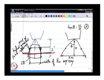
So, one way that imaging is often employed is if I take an edge of image of a spray let us say I take an image that is a sufficiently a large spatial representation of the spray cone angle. So, the liquid part is the liquid cone is very close to the nozzle here and then when I take the image I see all the missed and everything on the edge and if I take a line going across the spray and float the intensity in the image as a function of the position from the center line.
