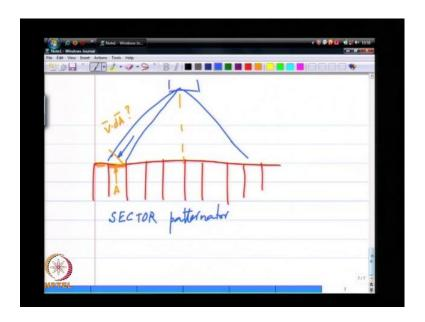
Let us make sure we understand this point if I did this same exact thing in an inline setting and I had a spray nozzle that is spraying, let us say I will intentionally draw a wide spray the collection going into this sector as a mean velocity in this direction which automatically means that, the collection area is not this area, but more like the area perpendicular to the velocity vector. So, essentially V dot d A, is what is responsible for the mass getting collected into the i-th chamber.
