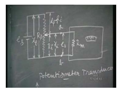
So the contact point will be moving up and down when we give the displacement of a machine number for example. So when the point is here, you will have zero, as the point moves up you will find the total voltage of  $e_s$  is distributed over the full length of the resistor. So as per the travel you will have you will have a voltage output. So at any instant the displacement is  $x_i$  and then accordingly you will have a voltage output.
