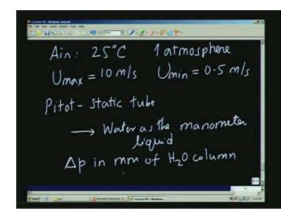
I will consider air as the flowing fluid at 25 degree Celsius, because the flow rate is dependent on the density, and I will assume that it is at a very small difference with respect to one atmosphere because delta p is there. The delta p is very small compared to the atmospheric pressure. The maximum velocity I know is about 10m by s, and the minimum velocity is about 0.5m by s this is the measured value, I am going to measure such values. In fact, I can find out what is the dynamic head.
