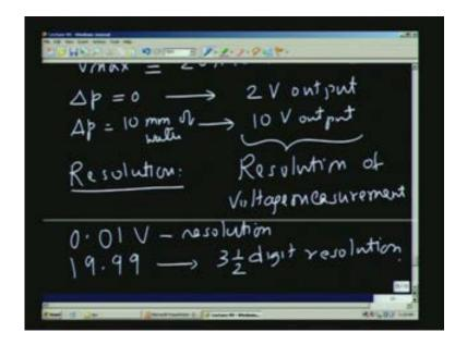
Suppose, for example, I am able to measure 0.01V resolution what does it mean?
