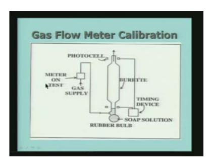
I have the meter on test, this may be any meter for example, a rotor meter and then I have gas supply it may be air in which case it will be air supply if
