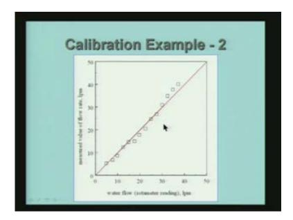
In fact, I have shown an example here. I am trying to calibrate a rotameter and essentially we have a similar set up and then the calibration looks as something like this. We have the measured value of the flow rate liter per minute and the water flow rotameter reading, the rotameter is calibrated and
