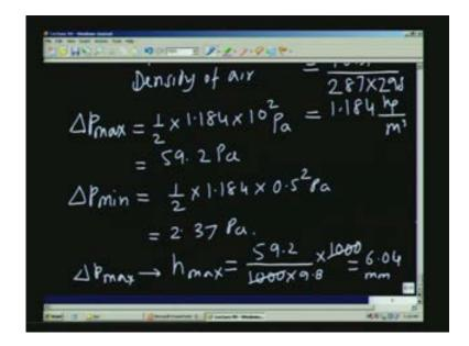
These two 1000 will cancel and you simply divide this by 9.8 and you get that value and that happens to be 6.043 mm of water. So the maximum we are going to measure  $h_{max}$  is 6 mm, and I can also calculate  $h_{min}$  it will be simply the value of delta p in Pascals 2.369 by 9.8 mm of water that will be 0.242 mm. Here we are talking about very small changes in h. So one option is to use a Betz manometer, where we use optical arrangement to measure delta h with a high degree of resolution.
