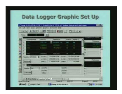
So in this case the channel is on and these four channels have been switched off. So what you see here is a virtual instrument in some sense of the system, because whatever is happening in each of this channel can be actually followed in real time. The next slide shows that how we setup the data logger for scanning the data. What is a scan? Because the data loggers have several channels, each channel has to be measured in a definite way.
