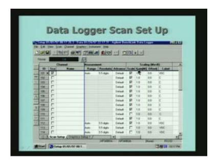
Suppose I have four channels, I cannot measure all the four channels at the same time so what the data logger will do is, it will go to one channel make a measurement go to the next channel make the measurement so a series of measurements will be made in time.
