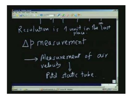
The primary instrument I am going to use is a pitot static tube. Let us find out the typical values of the velocities that are to be measured, and then accordingly we will find out the suitable instrument for that purpose of measuring the delta p.
