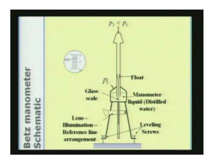
It is actually a well type manometer, we have a well here, that means it is a very large reservoir of water, I am going to use a liquid in the form of distilled water, and what I have is a tube which is sitting in the middle of that and the space above the well is connected to the higher pressure  $P_1$ , and the space above the column above this vertical tube is connected to the second pressure  $P_2$ , the lower value.
