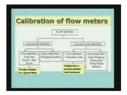
Let us see the schematic of how one goes about calibrating flow meter. We may have either gas flow meters or liquid flow meters, I am avoiding solid flow meters or solid flow. The gas flow meters can be either volumetric or it could be gravimetric, that means mass flow or the volumetric flow and liquid flow metric again you can have volumetric or gravimetric.
