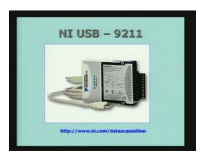
This is data acquisition. Data acquisition is one of the most important parts and National Instruments supplies a large number of data acquisition hardware accompanied with software. This is one of them; it is a national instrument USB. USB means it is going to be connected to the computer to the USB port. USB is nothing but Universal Serial Bus.
