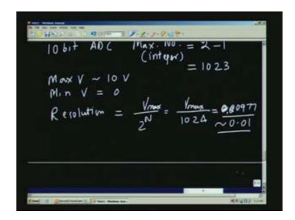
Actually we can make it exactly equal to 0.01, if I choose 10V a slightly higher value which will be just nothing but, if I take 10.24 you will see that it becomes exactly equal to 0.01. That means a 10-bit ADC can measure 10V in steps of 0.01V so that is the idea.
