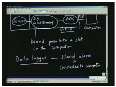
The connection in this case, is through USB. Earlier we used to have what is called, GPIB or General Purpose Instrument Bus, or it could be through a
