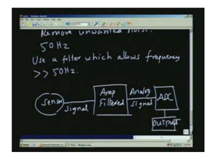
The output device may be a computer or may be digital voltmeter or whatever may be the type of instrument? So the input or the signal is analog and the output is digital, and this is communicated to an external device.
