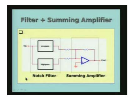
This summing amplifier is like what we showed a little while ago. And what you see is that the notch filter frequency response is like this. In this case of course, it is made for some other frequency and not for 50 Hz.
