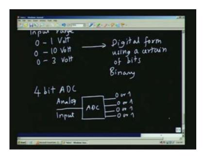
So, each one of these can be either 0 or 1. Of course, these can come in serial fashion or parallels as I have shown here. Now what we mean is that the each input is converted to an integer output. For example, if I have 4-bits the lowest bit is 2 to the power 0, 2 to the power 1, 2 to the power 2, 2 to the power 3 this is the 4-bit we are talking about. For example, I can have a
