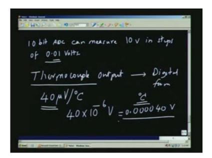
If you are going to convert a thermocouple output to digital form, for example, if you take thermocouple output to digital form, we know already that for a thermocouple, normally it is about, 40 microvolt by degree C. So if I want to resolve 1 degree Celsius, I need to sense 40 microvolt, here we
