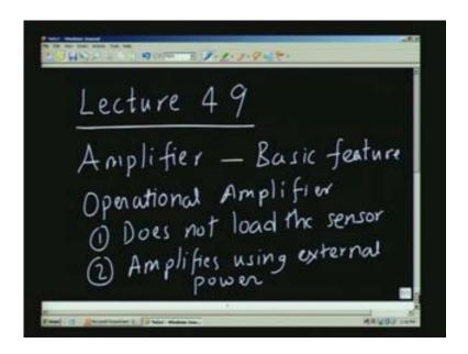
So, the operational amplifier is the heart of the signal conditioning system, and what the operational amplifier does is one does not load the sensor. So it draws no power from the sensor, or very little power from the sensor, amplifies the signal using external power. And in fact, I can represent the amplifier in a very schematic way as follows.
