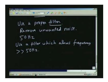
If I have an ac amplifier, and if I am looking at signals which are at sufficiently high frequency compared to 50 Hz then, I can use a filter which will remove the low frequency part of it and only pass the high frequency, so we have what is called a high pass filter. So, we can use a filter, which allows frequency much larger than 50 Hz. That means that the signal is also
