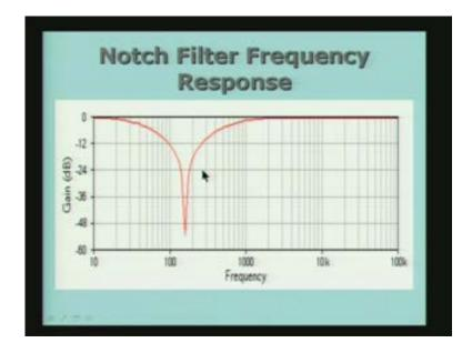
What you see here is that it allows the frequencies up to this and then at this particular frequency it blocks out completely. This is gain in db this is the logarithmic scale so it is attenuated to a large extent, therefore, this
