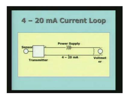
So you have a transmitter, and what the transmitter does is, it takes the sensor output and modifies it to a current proportional to the sensor output. If the sensor is a pressure measuring device, the pressure signal is converted to a current, and in this case if it is 4 to 20 mA that means that the maximum value of the current corresponding to 20 mA will correspond to the maximum of the pressure signal for which that pressure sensor is designed.
