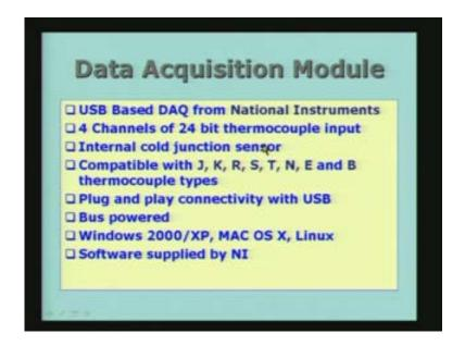
So just to see the resolution we are talking about, resolution of 1 by 2 power 24 is 5.96 into 10 power minus 8 it is something like approximately 0.1microvolt by V.
