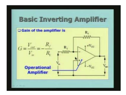
Therefore what the operational amplifier does is to give a magnitude give a gain which is purely determined by the resistance which we choose in this fashion here. We are talking about an amplifier and we just want to look at the basic features of an operational amplifier.
