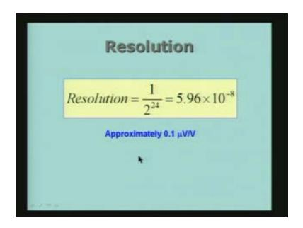
So you see that now we are talking about measuring very small voltage levels. Obviously, the instrument which I just now showed must have its own amplification, it must have its own manipulation, and all the items which we mentioned were already built into this 9211 so you do not have to connect anything specific to that, it is already there. And the software will take care of most of the things. And as I said earlier, the software which comes with National Instruments is the LABVIEW.
