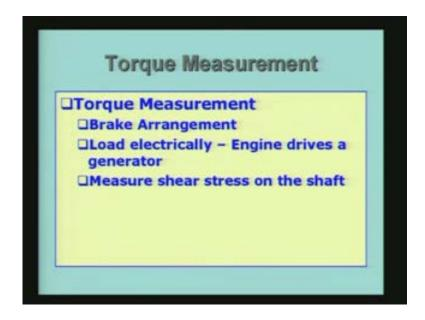
So I convert the mechanical power to electrical power and the electrical power is dissipated. And the more I dissipate the electrical power the more load it will bring on the engine therefore the engine load can be changed. And as the engine load changes we would like to find out what is the power developed and what are the characteristics. For example, I may be interested in finding out how much fuel it is consuming for a certain output.
