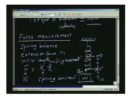
For example, I talked about spring balance. This is very commonly used. we have a support which is fixed and we a have spring and then we have the W, the weight which is hanging from it and you can put some kind of a pointer here attached to the base of the spring and you have a scale here. This is 0 and may be this corresponds to 10 so this is the weight.
