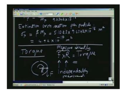
Because the errors in measurement of F and R are going to translate into error in the measured quantity that can be avoided it by measuring the torque directly. So why do we measure the torque? If you look at the following if you have rotating machinery, the torque multiplied by the angular velocity actually gives the power. So the reason why we are interested in measuring the torque is, of course, because we would like to measure the power through the same.
