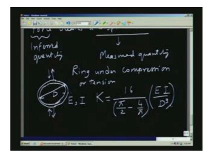
I am assuming that the ring is a small cross section compared to the diameter it is very thin therefore I will take this as the diameter and if you take the diameter of the ring and E the Young's modulus and I is the moment of inertia of the section about its central axis you can see what is going to happen.
