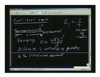
Again you see that the moment of inertia is going to determine, very clearly it is in the numerator, the longer the length the less stiff it is as you can see the length is in the denominator, and if we make it longer it becomes less stiff whereas if you distribute the material of the cantilever beam such that the moment of inertia is larger it is going to give you a larger spring constant.
