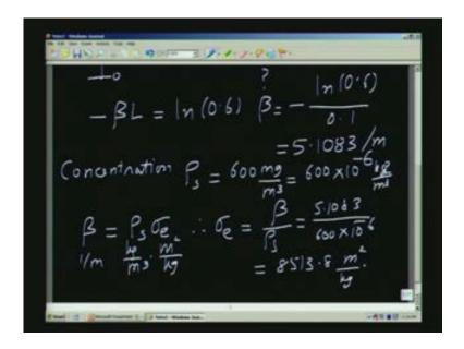
Here, everything is in SI units, so the extinction coefficient beta comes out to be 5.1083 m. This is per meter this is the first answer which is required. We also are given that the sample has got a concentration, so the concentration of the smoke, concentration is measured either in terms of the number of particles per cubic meter of the entire volume, or it could be amount of material per unit volume.
