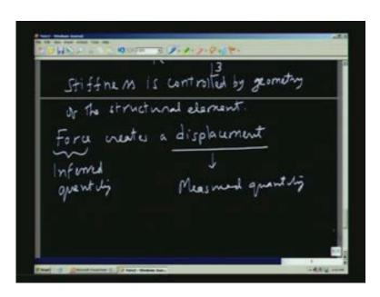
This actually is a transducer as you can see. You are converting a force into a displacement, and therefore it is a transducer. Let us look at one last element. It is in the form of a ring of material and you can apply the force either in this fashion or in this fashion. You can either compress or extend it. So it is in the form of a ring under compression or tension.
