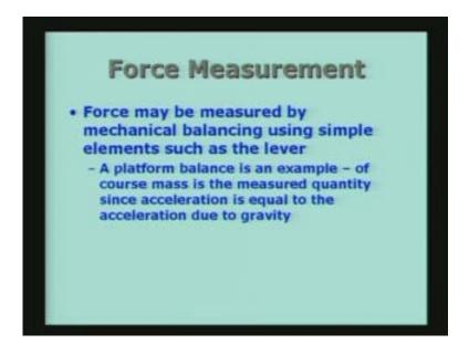
Let us now look at force measurement. So the force may be measured basically, by mechanical balancing using simple elements such as the lever. Force measurement can be done when it is not a dynamic situation. When the situation involves force measurement it could be through equilibration or when situation is one of equilibrium so you balance the force for example, the measurement of weight of a body or the mass of the body.
