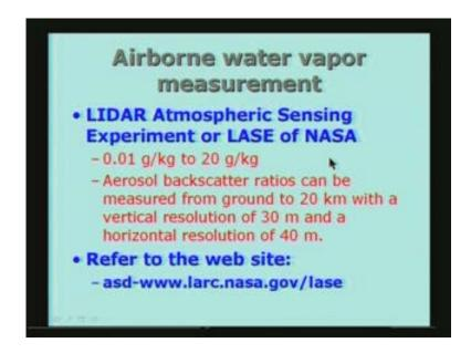
I can decide the particular region in which I want to make the measurement, and the resolution is 30m vertically and horizontal resolution of 40m. That means I can choose the region over which I can make the measurement. Here are a few characteristics:
