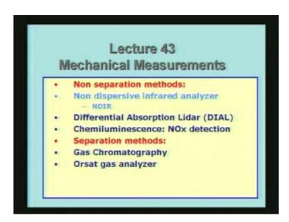
In fact, in the previous lecture we have covered already the non dispersive infrared analyzer, which is a very useful instrument which is used in day-to-day laboratory practice for measuring especially exhaust gases from IC engines. The second one I was trying to describe in some detail was the differential absorption Lidar. Lidar stands for light detection and ranging and the particular technique is called dial or differential absorption Lidar.
