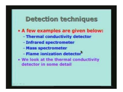
Therefore different detection techniques are possible. Here are a few examples. For example, here is the thermal conductivity detector. I can use the infrared spectrometer. We discussed about spectrum of various gases, they have specific bands in which they will absorb therefore if you use an infrared spectrometer by finding out where the absorption is taking place, I know what gas it is and also by measuring the amount of absorption I can immediately say what the concentration is.
